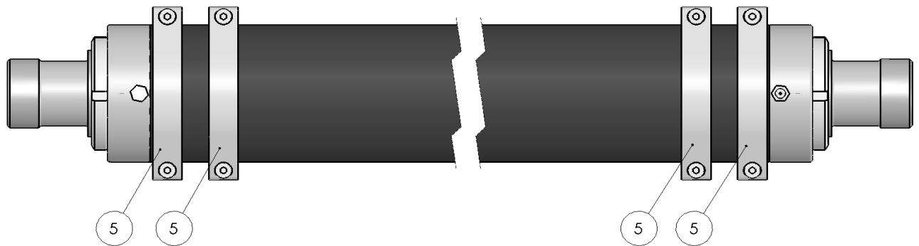
Figure 17. Installing the pulsation hose flange and hose clamps.
