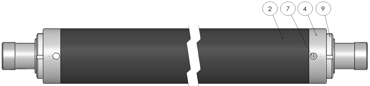
Figure 16. Installing the cover hose.
