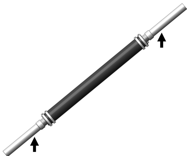
Figure 6. Pipeline supports in angled installation.
