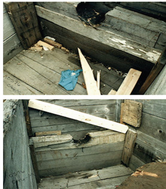
Figure 17 – Damage may occur due to improper packaging during transport.
