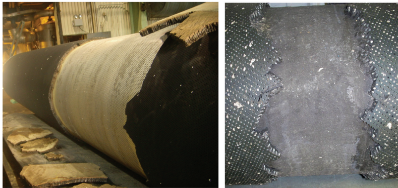
Figure 9 – Examples of localized overloading of rubber covers
