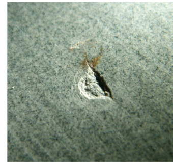
Figure 7 – Example of impact damage to ceramic roll
