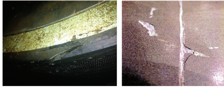
Figure 16 – Examples of roll cover damage which occurred during handling
