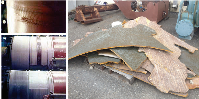
Figure 10 – Examples of localized overloading of polyurethane covers
