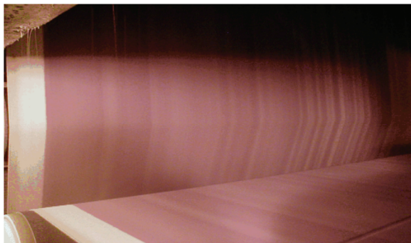
Figure 2. Poor center roll doctoring combined with this severely streaky bottom press wet felt to create sheet quality problems.
