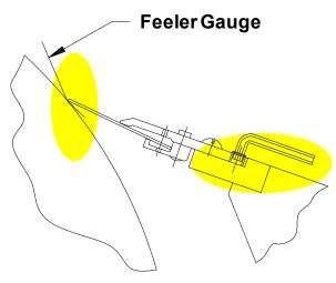
Figure 12. A feeler gauge can be used to profile a holder.
