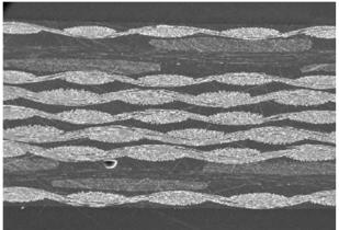
Figure 7. Cross section of carbon fiber blade, 2 layers of carbon and 5 layers of glass fiber
