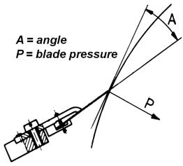
Figure 13. Blade angle and pressure
