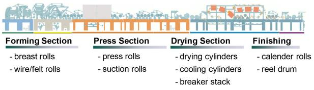
Figure 16. Doctoring positions on the machine
