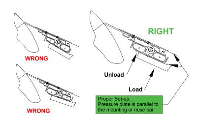
Figure 9. When setup correctly the pressure plate is parallel to the mounting or nose bar.
