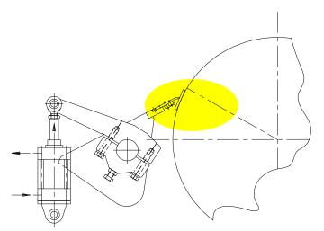
Figure 8. Adjusting safety distance KF-Holder and roll surface
