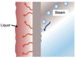
Figure 4. Falling film evaporation
