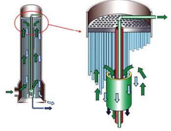
Figure 9. Internal condensate segregation
