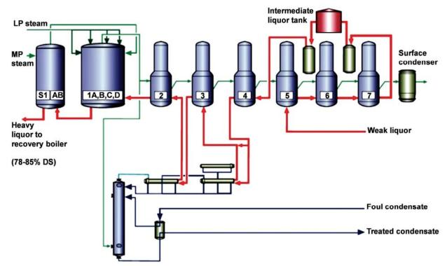
Figure 3. Simplified flow sheet for modern evaporators
