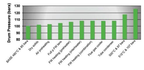
Figure 20. Cumulative effect of high power features on drum pressure (FW = feedwater).
