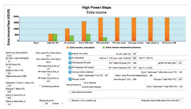
Figure 24. Extra yearly income from increased electricity produced by high power features (Case study #2).
