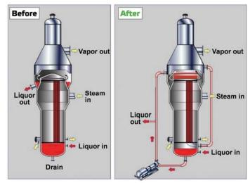
Figure 5. LTV to falling film conversion
