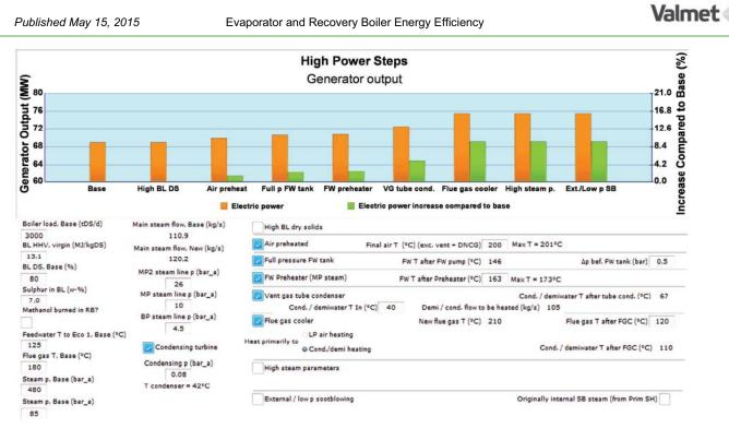
Figure 21. The effect of high power features on electricity production (Case study #1).
