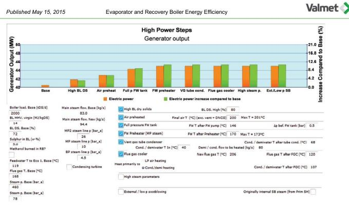
Figure 23. The effect of high power features on electricity production (Case study #2).
