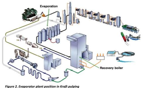
liquor leaving the pulp washers to a sufficient concentration to allow firing and combustion of the liquor in the recovery boiler.
