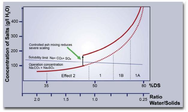
Figure 8. Ash addition prior to final concentration
