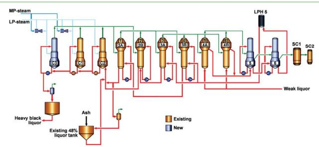
Figure 14. Eastern US mill revised evaporator arrangement
