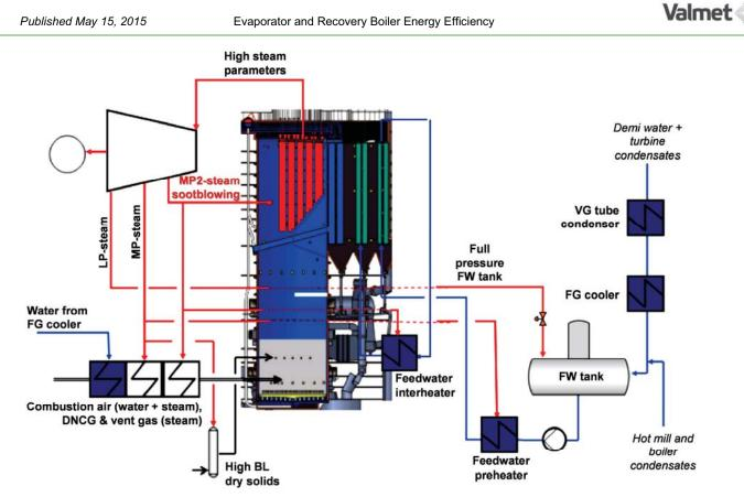
Figure 15. High power features in recovery boilers
