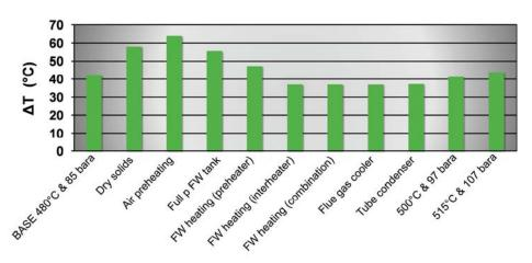
Figure 18. Cumulative effect of high power features on temperature difference between drum and SWC (SWC = sweet water condenser; FW = feedwater).
