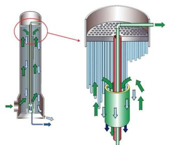
*Figure 9. Valmet's shell side design improves condensate segregation.*
