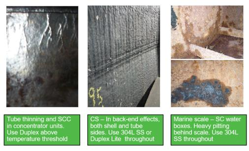
Figure 6. Three main areas of corrosion in evaporators. SCC in the SS concentrator bodies, general corrosion and thinning in the CS back-end bodies and marine scale in the CS water side of the surface condenser.
