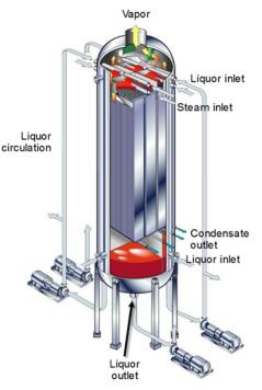
Figure 2. The TUBEL concentrator addresses scaling.
