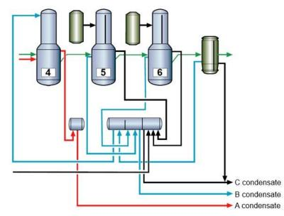
Figure 10. Valmet's ICT processes a portion of the B-Condensate to make A-Condensate in the shell side of the 4th Effect.
