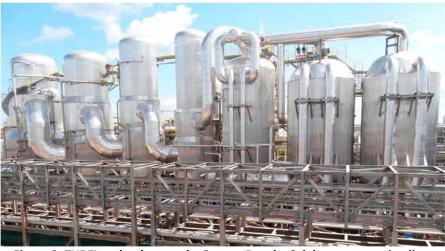
Figure 3. TUBEL technology at the Suzano Papel e Celulose evaporation line
