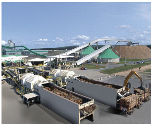
Figure 1. An example of a gentle wood conveyor feeding the debarking process
