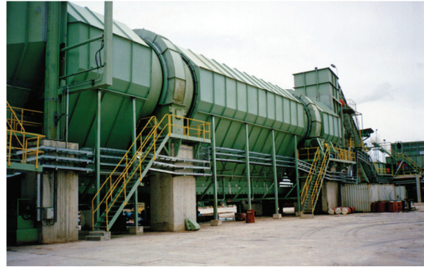
Figure 9. The EasyFloat debarking drum is hydrostatically supported and provides optimal bark removal with minimum wood loss.
