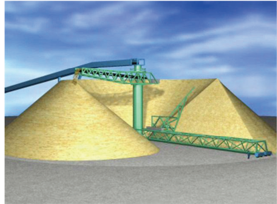
Figure 25. The GentleStore chip storage system builds the chip pile from the front and reclaims from the back, across the entire cross section of the pile.
