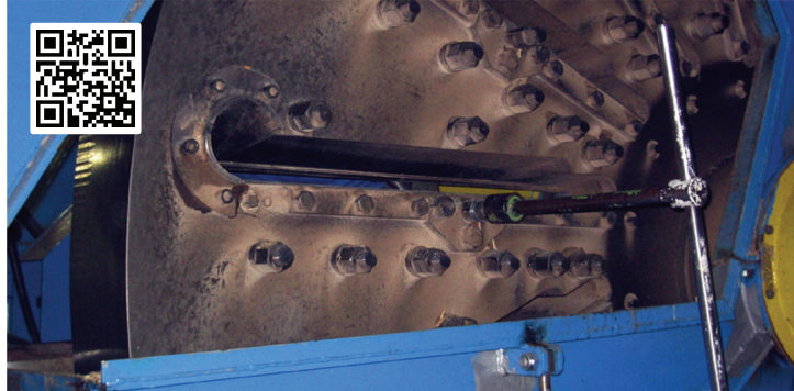
Figure 17. The QuickLock knife fastening system saves time. The one-bolt system requires only 15 minutes to change 15 knives, compared to 50 minutes for a traditional system with turntable knives.
