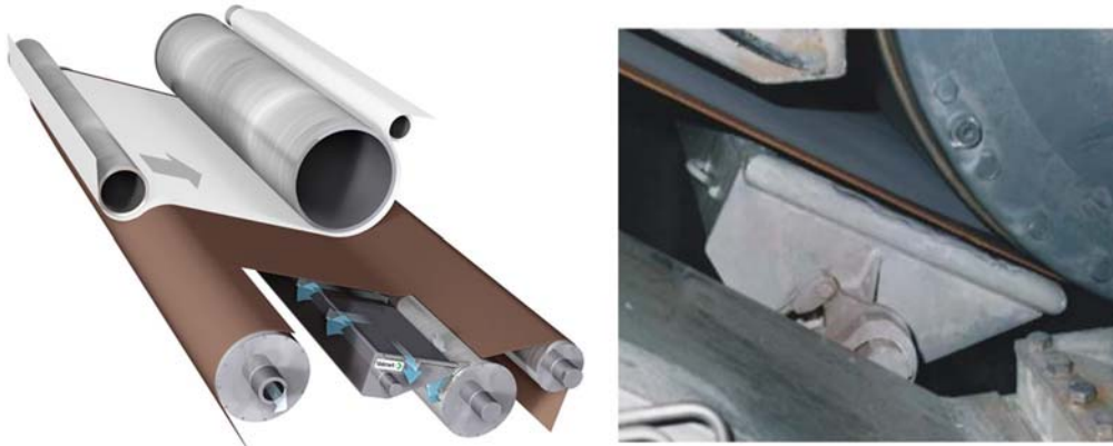
Figure 10. The Valmet Press Nip Web Stabilizer prevents an air bubble in the nip.
