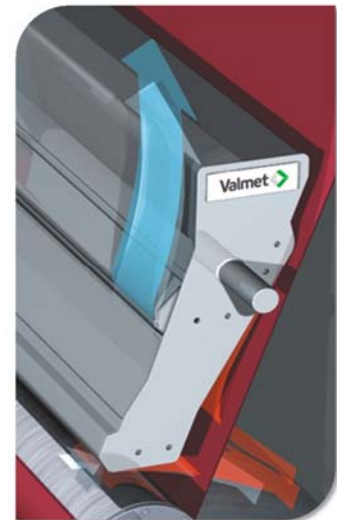
Figure 18. The Valmet Dryer Pocket Ventilator TR concept is for medium to high speed machines with special double-felted arrangement. The geometry for the concept is different compared to normal double-felting. Pocket rolls are placed non-centrally toward the wet end. The sheet is supported onto the fabric by utilizing the blow box principle in combination with the pocket ventilator principle.
