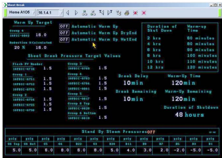
Figure 34. The Sheet Break screen allows operators to monitor and control all essential drying process variables during automatic operations.
