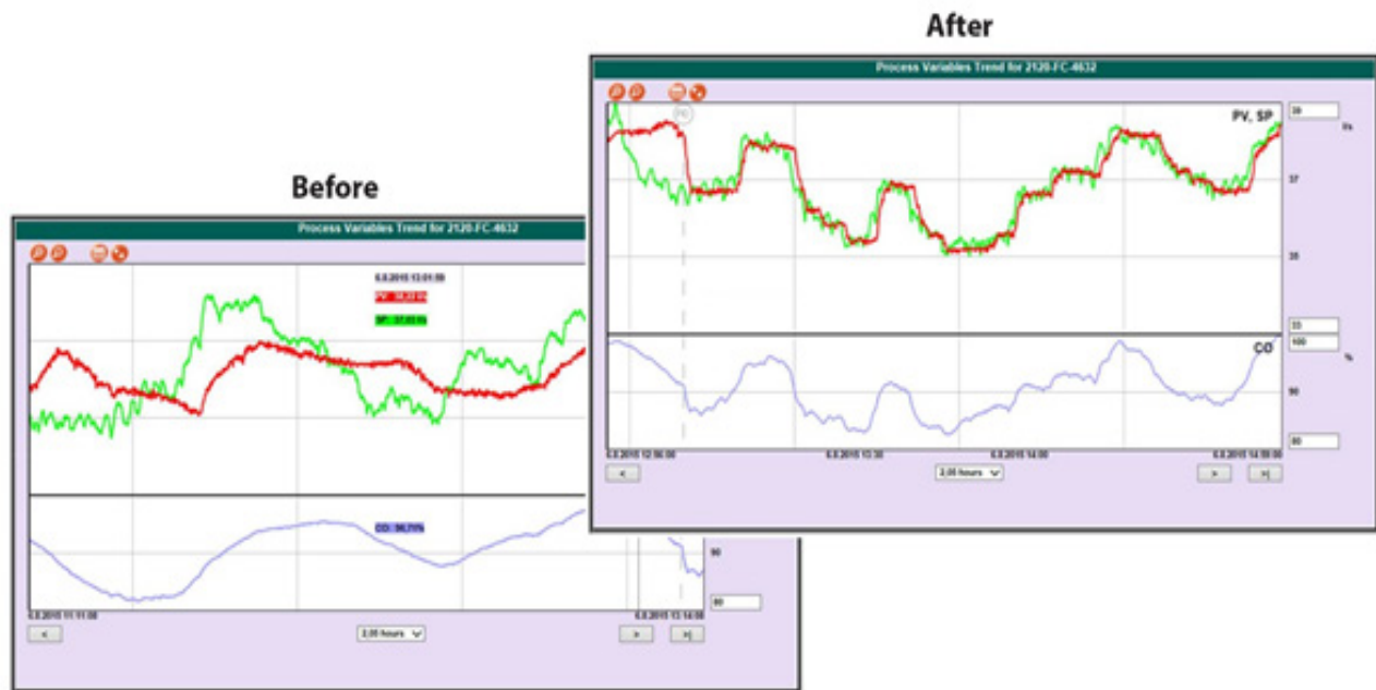
FIGURE 1: Controller tuning is a simple, non-invasive action that can lead to significant improvements. In this chart, the process variable (red line) is supposed to follow the green Setpoint line. With the old tuning, the control was sluggish and unresponsive. The simple tuning correction ensures that the plant is quickly performing exactly where it should be.
