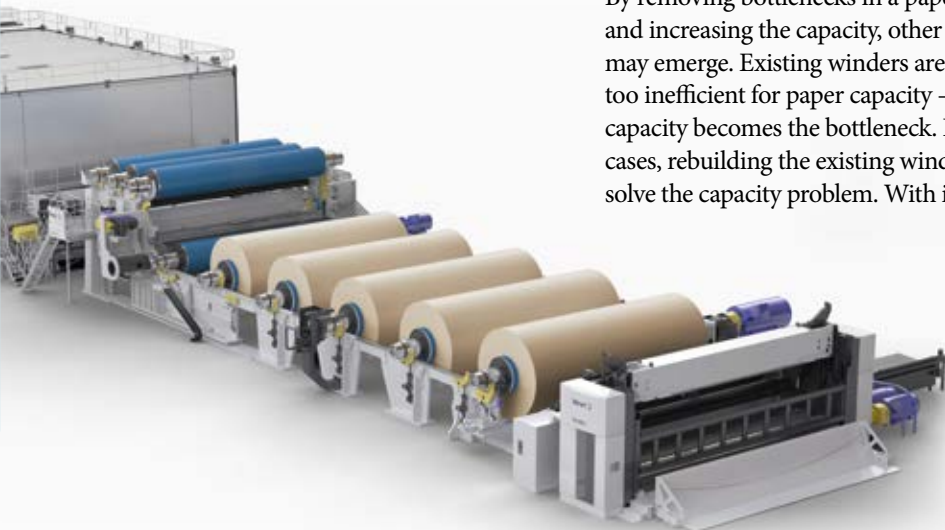
The OptiWin Drum winder (formerly known as WinDrum Compact) at Greenpac Mill is designed and constructed according to ISO 13849-1. The Occupational Safety & Health Administration (OSHA) adopted the machine guarding-related part of this standard in 2012.
