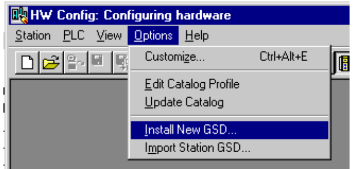
Figure 2. Install New GSD.
