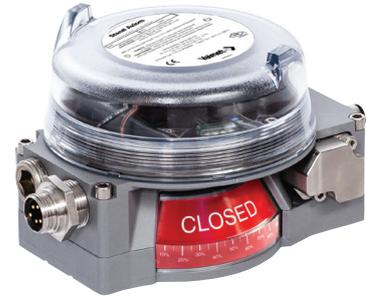
The Axiom™ provides advanced monitoring and control in explosionproof, non-incendive, intrinsically safe and general-purpose applications. It is a discrete on/off valve controller with proximity switches for quarter-turn automated valves. Its rugged construction will withstand the most challenging plant environments.
