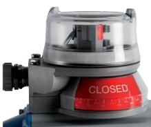
**QN:** Nonincendive is approved for Div. 2/Zone 2 hazardous environments with proximity sensors using a clear cover. Intrinsically safe Namur sensors or passive switches are available for Div. 1/Zone 0 applications.
