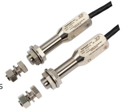
The explosionproof Hawkeye, with its stainless steel enclosure, is designed for service in harsh process environments. It features a solid state proximity sensor which is encased in a shock absorbent urethane potting material. Outputs for universal switching or NAMUR (EN 60947-5-6; I.S.) are standard options.
