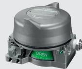
The stainless steel version of the explosion proof Axiom ANX is an optimum solution for standard on-off applications. It is a discrete on-off valve controller that combines a solenoid valve and proximity switches into one integrated package. The advanced position sensing system of Axiom offers reliable long-life performance with convenient push-button settings. The internal pneumatic valve has high tolerance to dirty air and it enables perfect operation in demanding off-shore environment.
