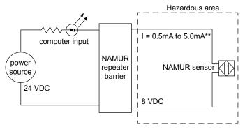
\*\* Barrier off state (target off): current in NAMUR sensor circuit >2.1 mA Barrier on state (target on): current in NAMUR sensor circuit <1.0 mA
