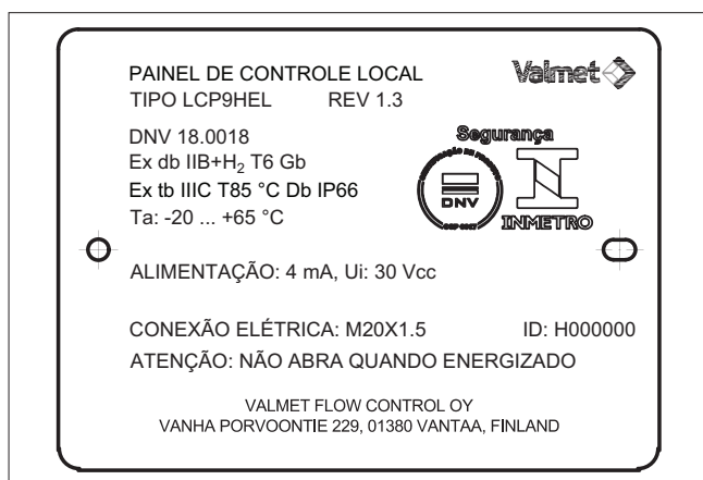
Fig. 3 Example of identification plate, LCP9HE
