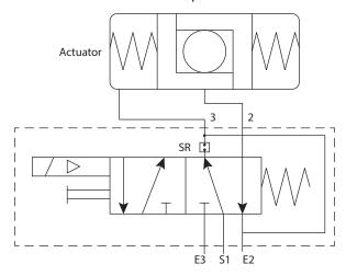
Fig. 2 Single pilot spring return pneumatic valve on doubleacting actuator with rebreather closed
