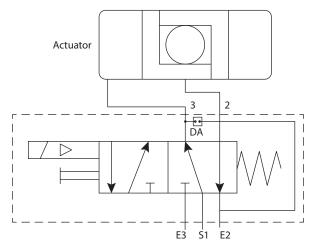
Fig. 3 Axiom dual coil shuttle piston pneumatic valve
