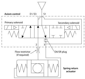
Fig. 5 Expeditor pneumatic valve on double-acting actuator
