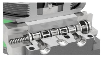
The Axiom's pneumatic valve system consists of a low-power pilot that drives the main high-flow spool valve. Pilots may be selected for conventional or bus networking applications. Both stages of the pneumatic valve system have been designed for long life, high tolerance to air line contaminants, and ease of maintenance should components become fouled. Pilots are automatically associated with the appropriate function selected.
