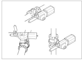
Fig. 7 Ways to install the actuator
