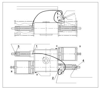
Fig. 23 Valve is open, operation to closed position
