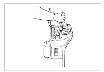
Fig. 16 Removing hydraulic cylinder piston rod
