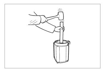
Fig. 19 Placing the piston in the cylinder
