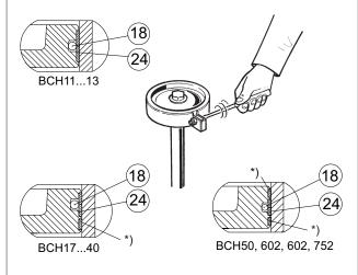
Fig. 18 Tightening the piston seals with a tie ring
