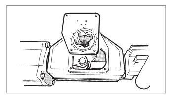
Fig. 20 Mounting the cover on the housing
