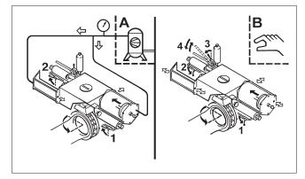
Fig. 15 Operating instructions plate for BCH502, opening the valve
