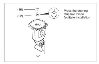
Fig. 17 Mounting the piston rod bearing and seal
