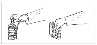
Fig. 22 Dismantling the linkage
