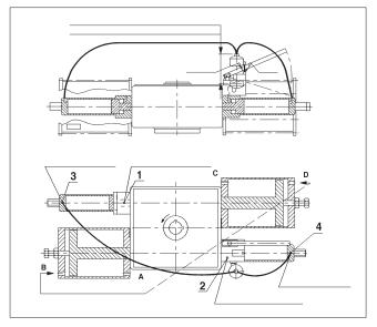
Fig. 24 Valve is closed, operation to open direction
