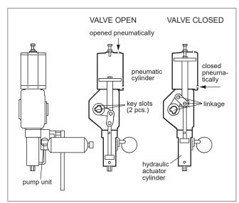
Fig. 1 Operating principle of the B1CH and BCH actuators
