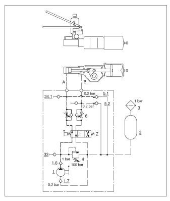
Fig. 12 Operating principle of the hydraulic pump unit on manual control, operating to closed position
