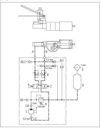
Fig. 11 Operating principle of the hydraulic pump unit on remote control
