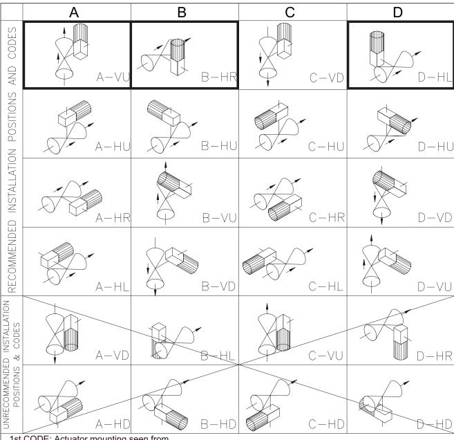
1st CODE: Actuator mounting seen from the upstream side (in unidirectional valves). In bidirectional valves seen from the upstream side in the piping dwg.
