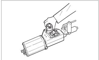
Fig. 21 Removing the linkage from the housing
