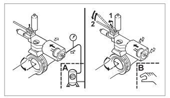
Fig. 13 Operating instructions plate, opening the valve
