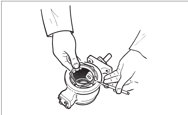
Fig. 16 Mounting the seat
