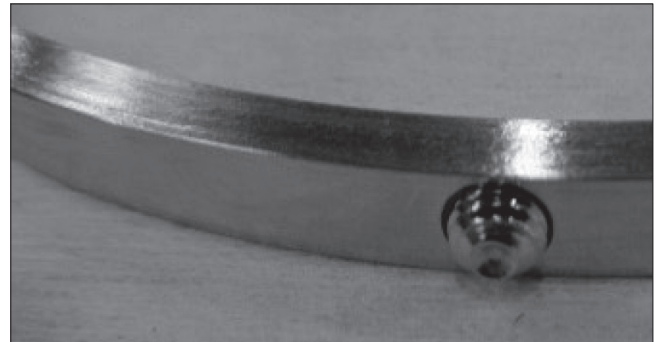
Fig. 19 Inside retainer (310) with (not yet finally) inserted grub screw (313)
