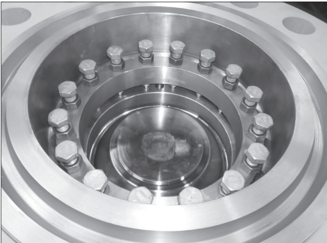
Fig. 18 Valve in CLOSED position
