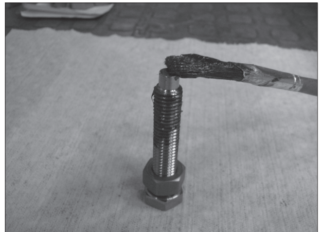
Fig. 26 Lubricate the screws with Molykote
