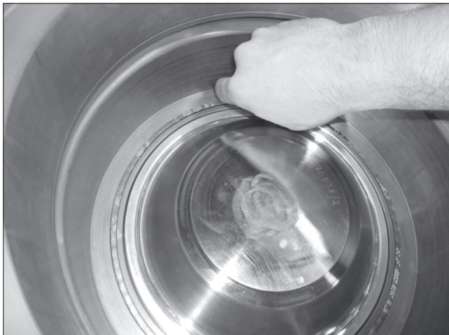
Fig. 23 Remove the sealing ring (304)
