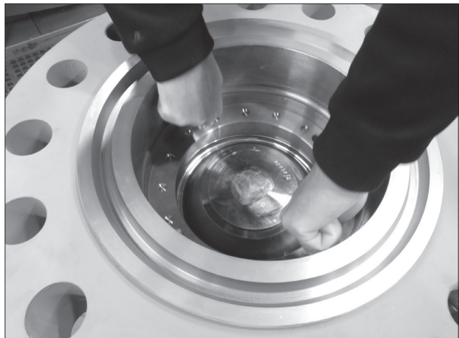
Fig. 20 Demount the retaining ring (301)
