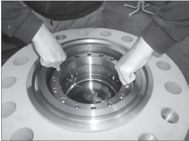
Fig. 22 Remove the inner seal lock ring (301)
