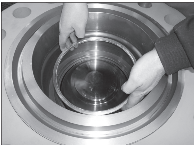
Fig. 24 Replace the metallic seat ring (321)
