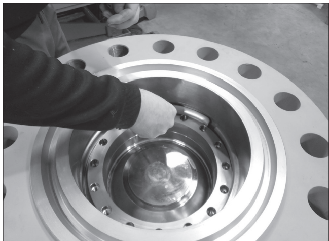
Fig. 21 Remove the outer seal lock ring (303)
