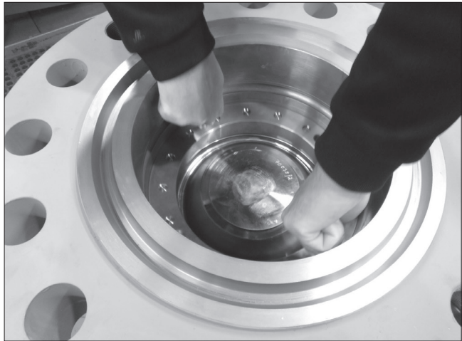
Fig. 20 Demount the retaining ring (301)
