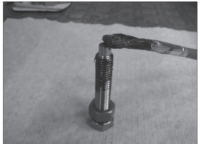
Fig. 26 Lubricate the screws with Molykote
