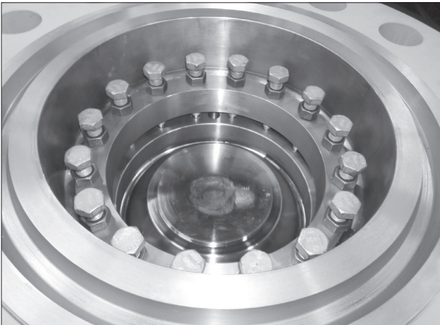
Fig. 18 Valve in CLOSED position
