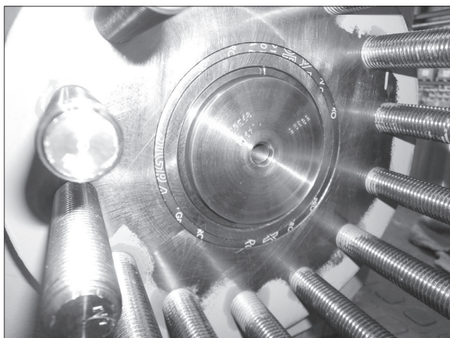
Fig. 30 Remove the graphite sealing ring (470)
