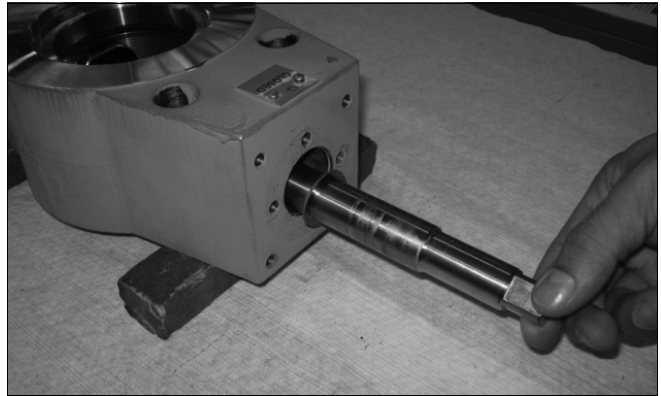
Fig. 58 Pulling out the shaft
