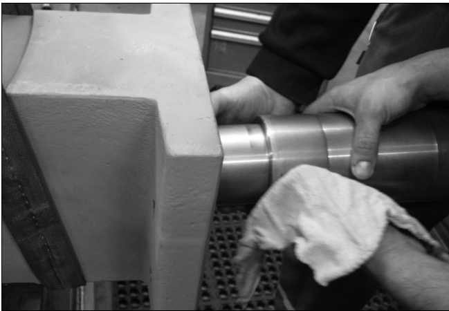
Fig. 47 Pulling out the shaft
