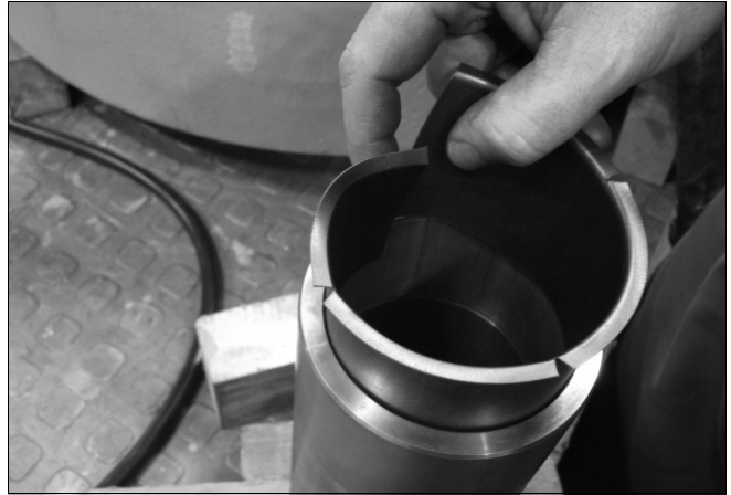
Fig. 49 Replacing the Metaloplast bearing
