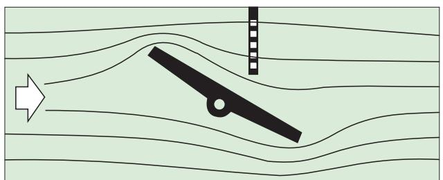
S-DISC design offers stable flow control, reduced dynamic torque, noise level and vibration. For more information see technical bulletin 2SL120.
