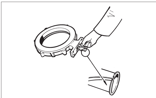
Fig. 16 Mounting the standard bearings
