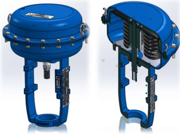
VDD - Direct Acting Spring to Open / Air to Close
