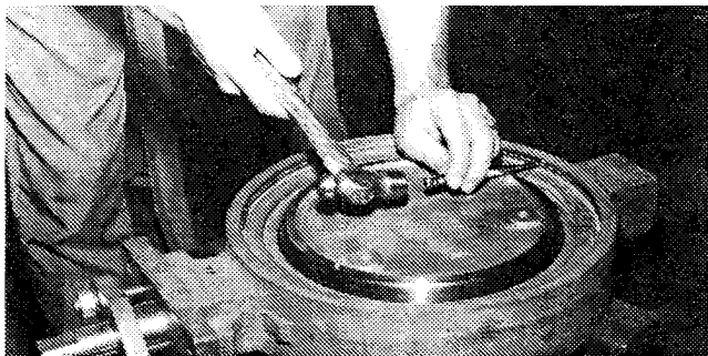
Tapping End Of Spring Into Body
