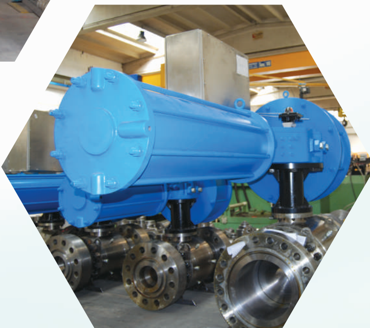
Gas over oil for Gas pipeline
