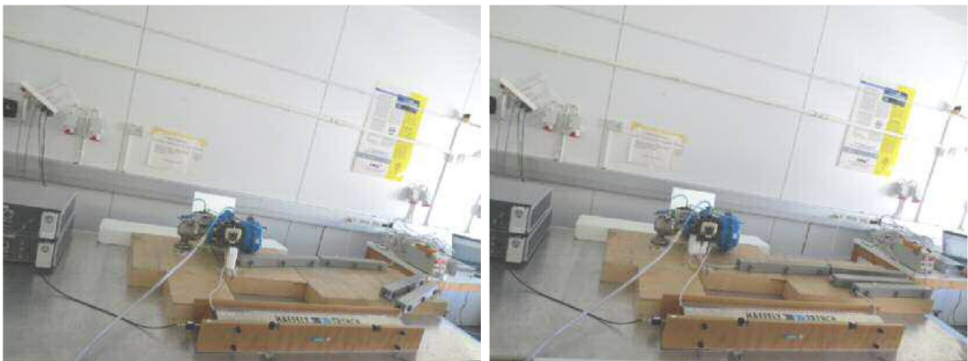
Photograph 10. The EUT and test set-up for electrical fast transient immunity.
