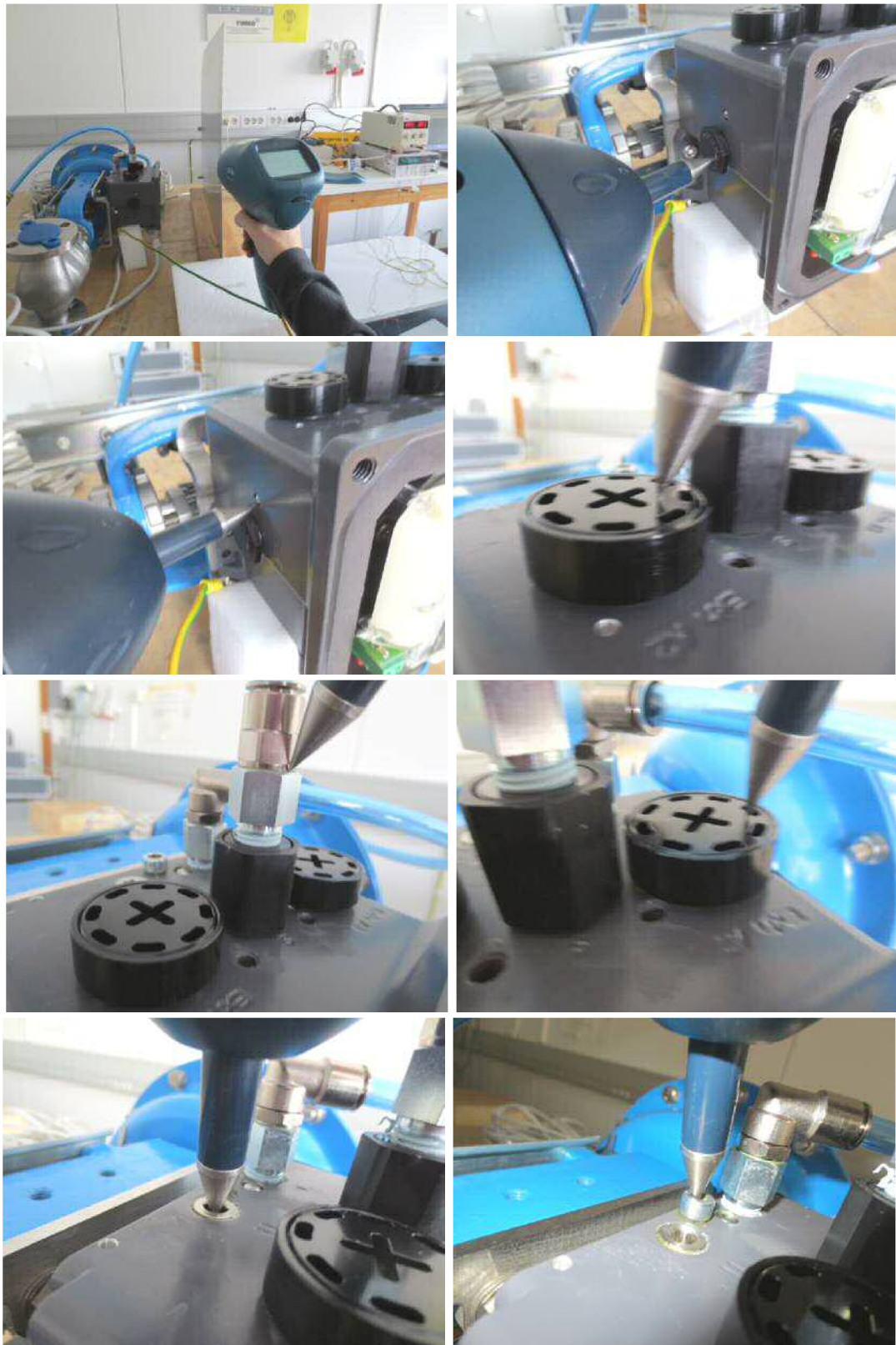
Photograph 6. The EUT and test set-up for electrostatic discharge immunity.
