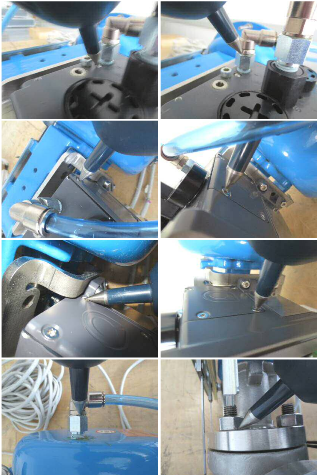
Photograph 7. The EUT and test set-up for electrostatic discharge immunity.
