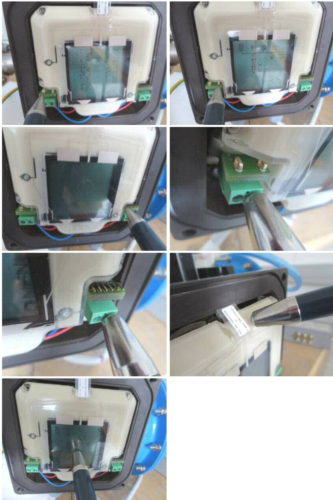
Photograph 8. The EUT and test set-up for electrostatic discharge immunity.
