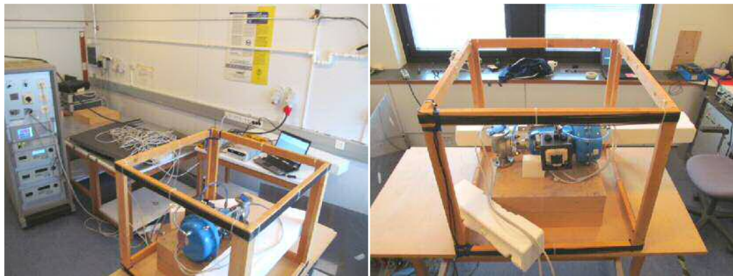
Photograph 13. The EUT and test set-up for power frequency magnetic field immunity.
