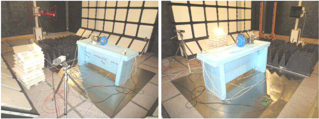
Photograph 9. The EUT and test set-up for radiated RF-field immunity.
