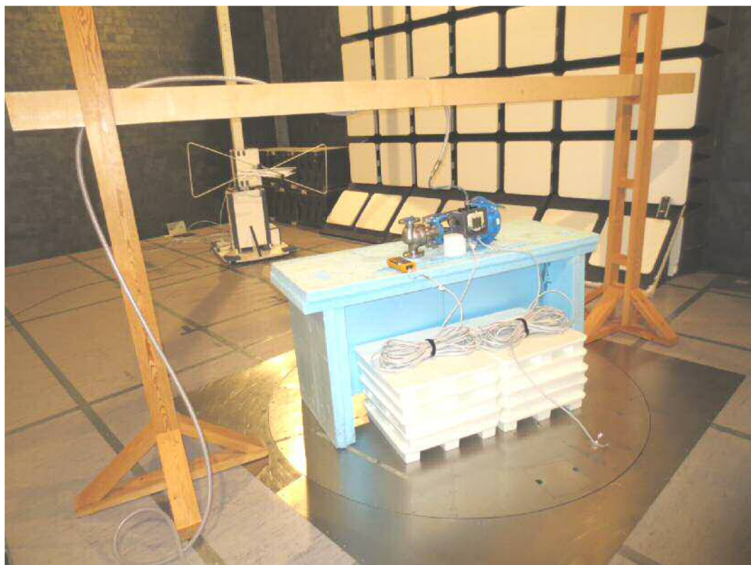
Photograph 4. The EUT and test set-up for radiated emission test
