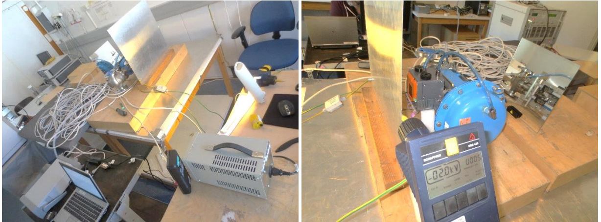
Photograph 5. The EUT and test set-up for electrostatic discharge immunity.
