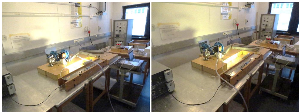
Photograph 13. The EUT and test set-up for electrical fast transient immunity.
