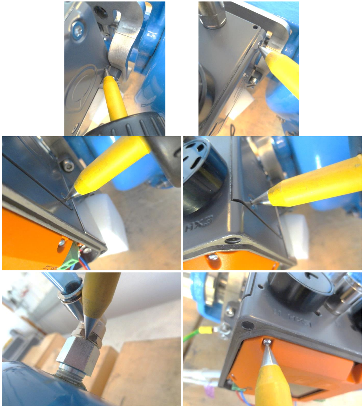
Photograph 8. The EUT and test set-up for electrostatic discharge immunity.
