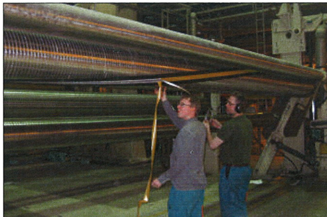
5. Installation of portable measurement sensors on a roll surface.
