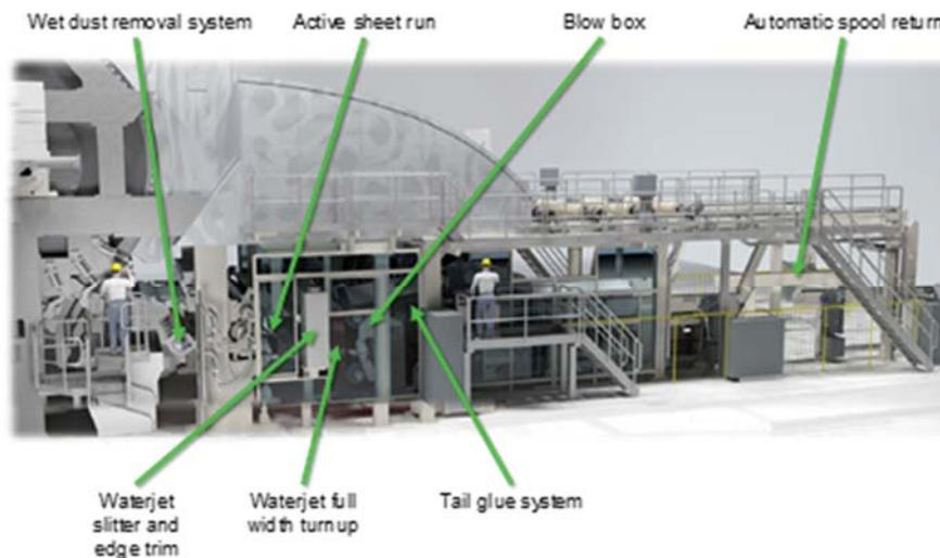
**Figure 15. State-of-the-art dry end layout with belted reel**
