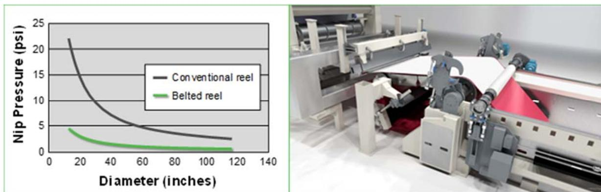
**Figure 8.** Nip pressure in a conventional reel vs. the belted reel. Belted winding provides a better start, with only 1/5 of the nip pressure required by conventional reels. Lower nip pressure preserves bulk.
