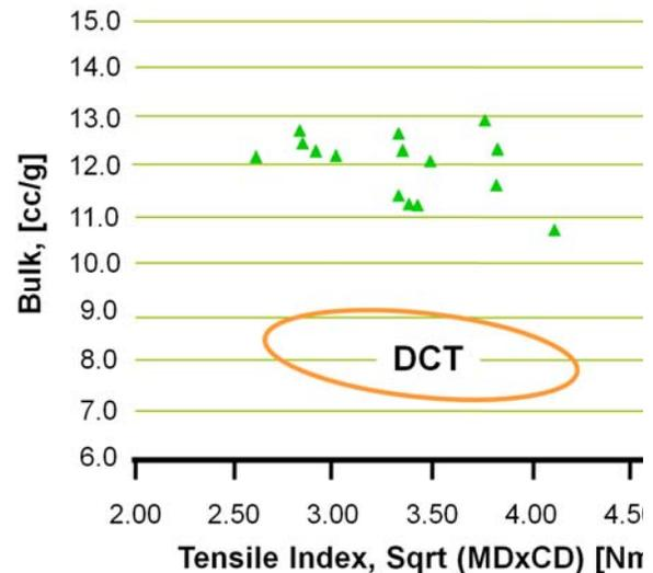
Figure 2. Bulk vs. Tensile Index (toilet tissue 18gsm)
