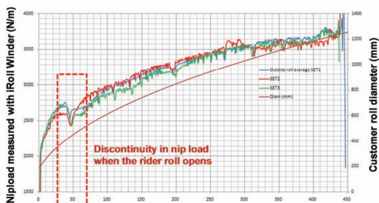
Figure 23. On-line condition monitoring of the winding nip with iRoll Winder provides instantaneous insight into winding irregularities.
