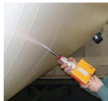
Figure 21. The Schmidt hammer test is typically used to measure roll hardness, but is a manual offline process.
