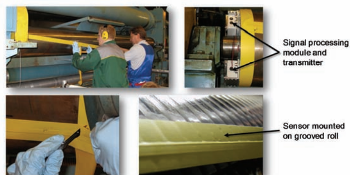
Figure 2. Valmet technicians install the iRoll Portable sensors on-machine in the mill.
