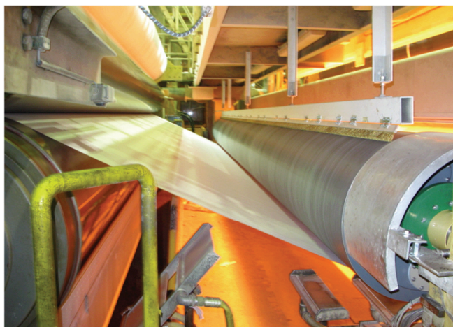
Figure 1. iRoll installed in a tension measurement application.
