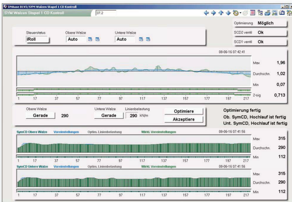
Figure 9. iRoll measurement and control operator interface as used on Plattling-Papier PM1
