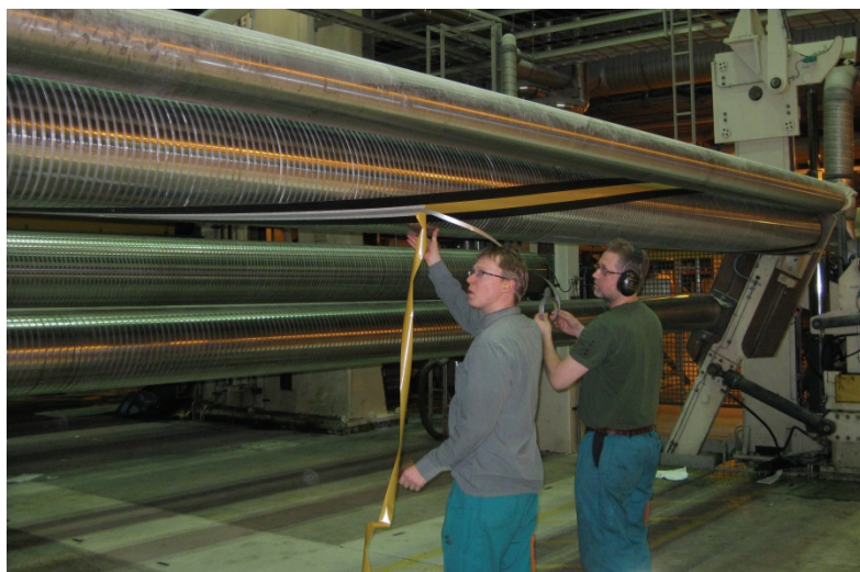
Figure 5. Installation of portable measurement sensors on a roll surface.
