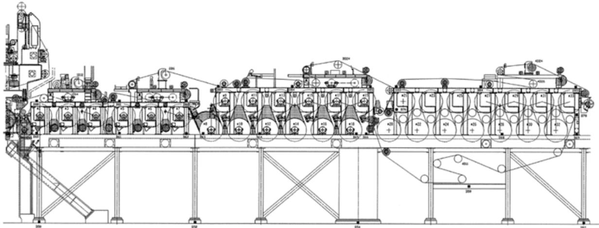
Figure 4. Dryer section after reinforcements installed.
