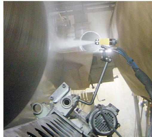
*Figure 9. Valmet Dryer Roll Cover DOH release coating is well-suited for onsite application.*
