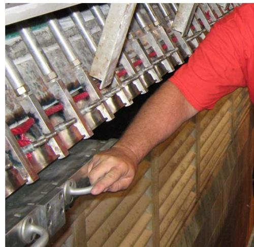
*Figure 14. Valmet technicians can repair minor damage to your apron edge, grind, and then polish it to like-new condition. And, it can all be done on-site with the apron in the machine.*
