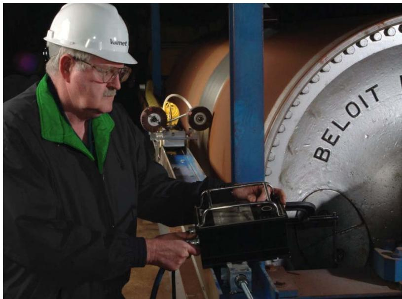
*Figure 8. Valmet can apply multiple crews and tools to a dryer resurfacing project to increase the number of dryers that can be cleaned in one shutdown.*
