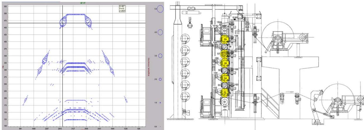
**Figure 12. Vibration map (left) and supercalender showing filed rolls (right, yellow). A relatively simple software change resolved this difficult operational problem.**
