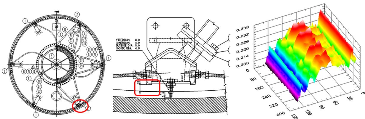
Figure 10. This vibration problem was solved by increasing the distance between the Yankee rib and condensate header.
