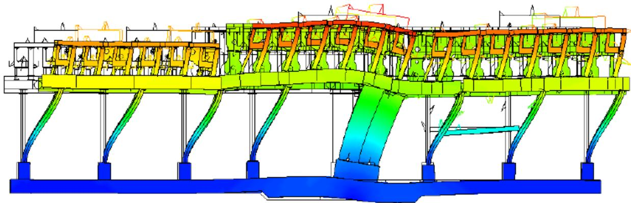
*Figure 3. Dryer section modeled with Finite Element Analysis, showing expected deformation at target frequency of 3.52 Hz.*
