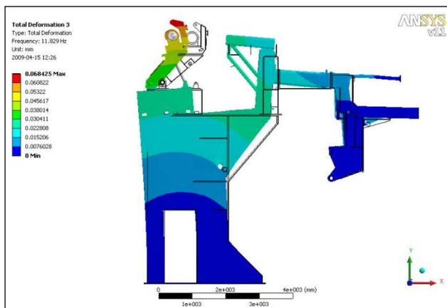
**Figure 11. Solving this vibration problem required creating a computer model of the stretcher roll and framing.**
