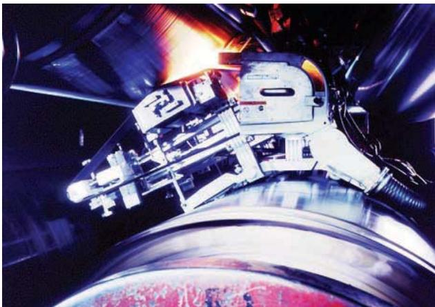
*Figure 7. Dryer Profile Grinding is performed onsite and results in a flat CD dryer profile.*
