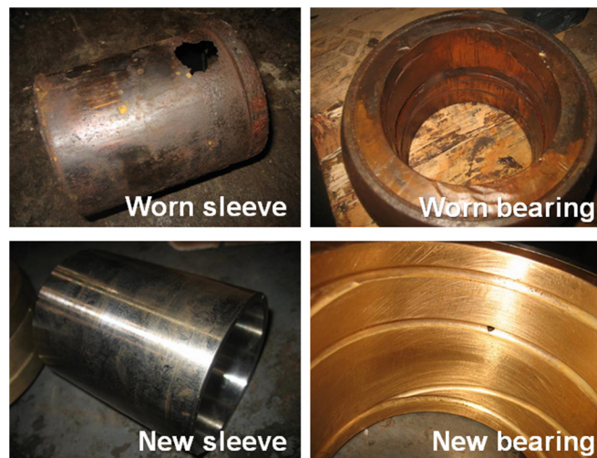
Figure 15. Center roll doctor beam bearings, worn vs. new
