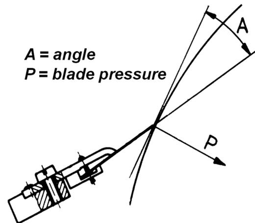
**Figure 13. Blade angle and pressure**
