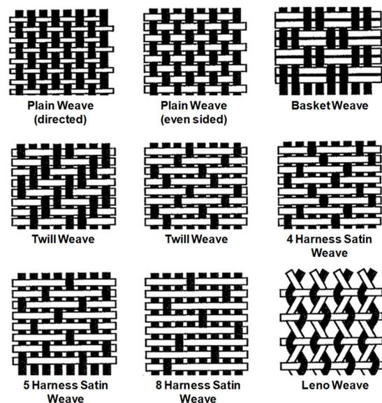
Figure 4. The most common fabric binding structures
