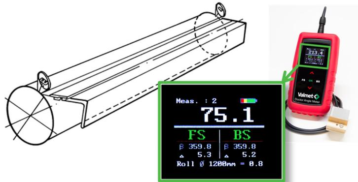
**Figure 10. Aligning a doctor using the Valmet BladeAngle tool.**
