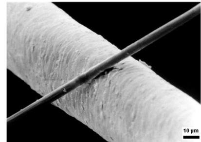
Figure 3. Carbon fiber vs. human hair (black fiber is carbon fiber)
