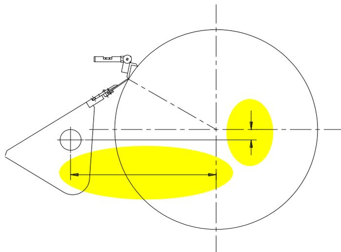
**Figure 11. Aligning a doctor using a bubble gauge**
