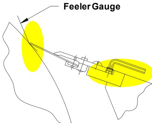
**Figure 12.** A feeler gauge can be used to profile a holder.
