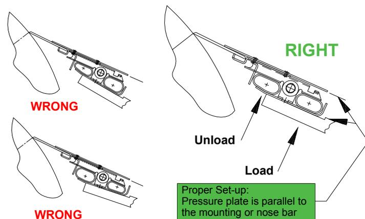
Figure 9. When setup correctly the pressure plate is parallel to the mounting or nose bar.
