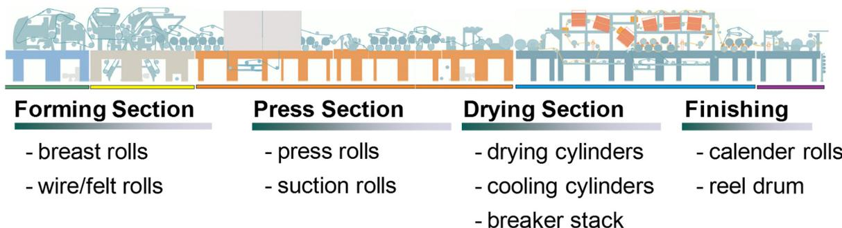
Figure 16. Doctoring positions on the machine
