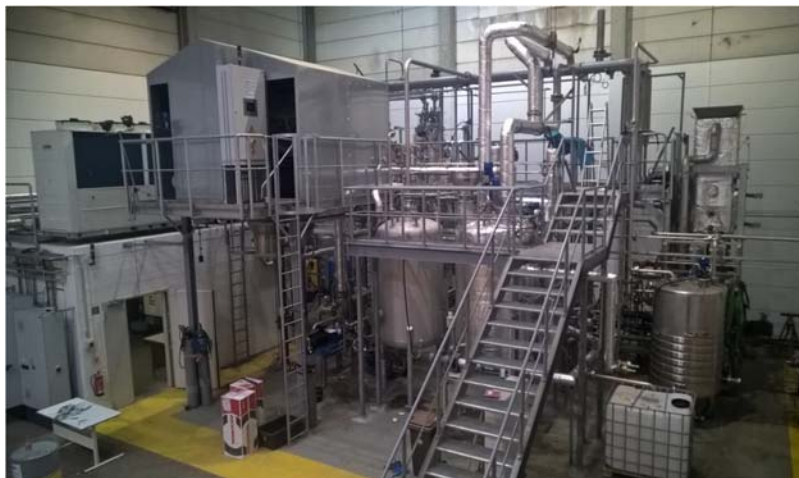
Figure 5 Hydrothermal carbonization pilot where lignin experiments have been carried out
