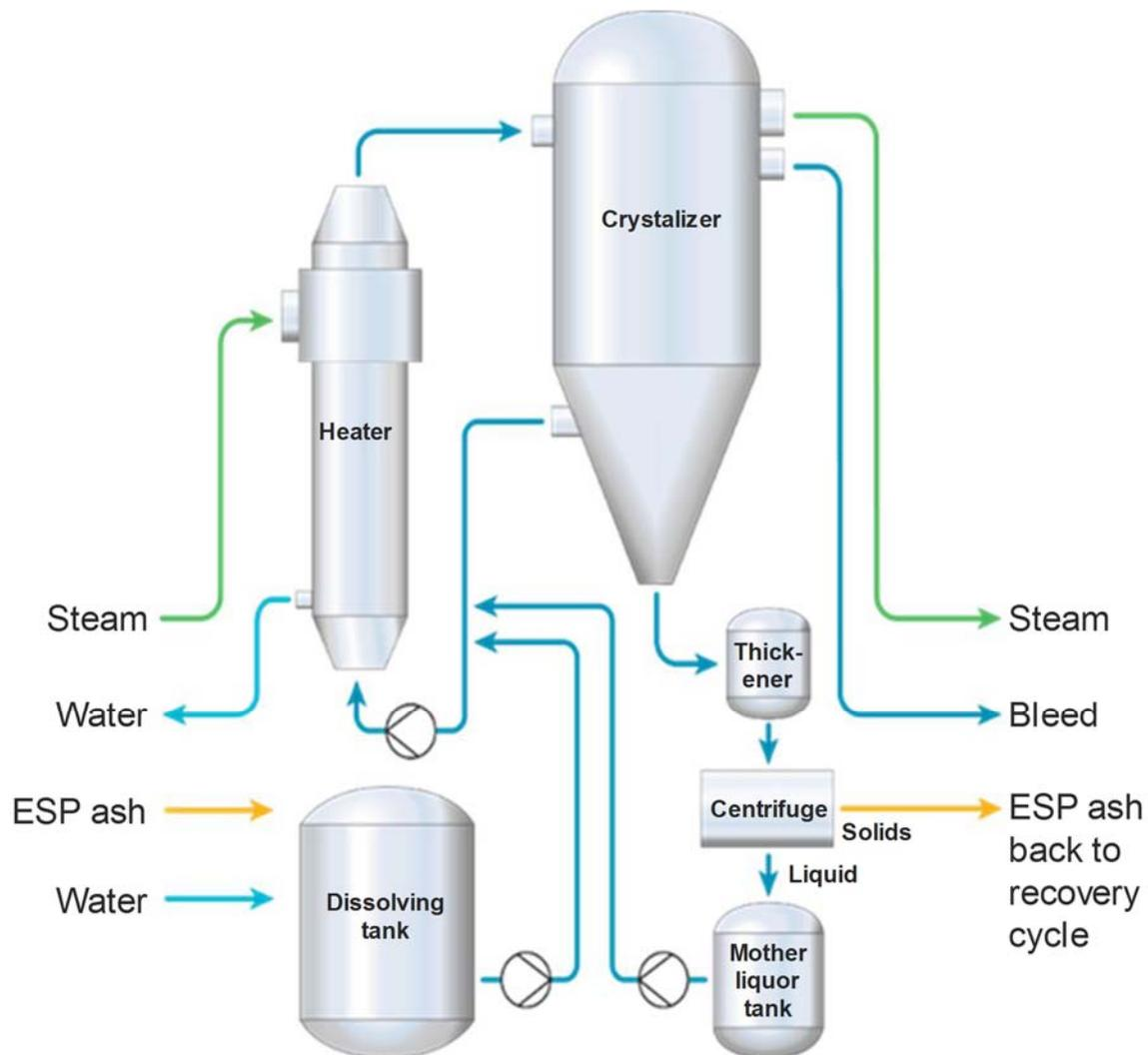
**Figure 10. Crystallizer operation principle**
