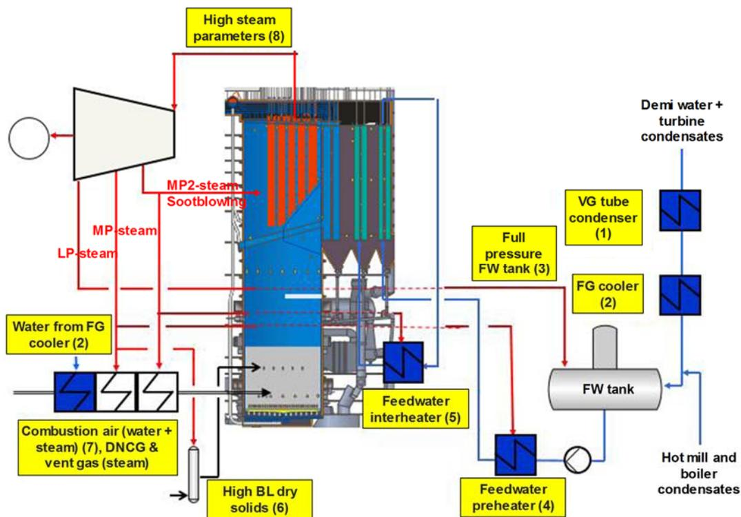
**Figure 2. High power features in recovery boilers**
