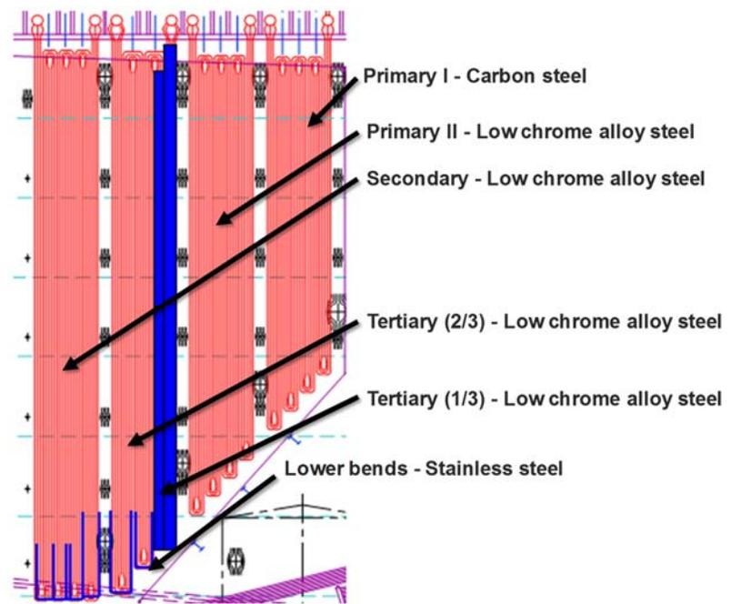
**Figure 6. Typical amount of stainless and carbon steel in superheaters**
