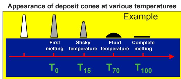
**Figure 4. Ash melting deformation temperature**
