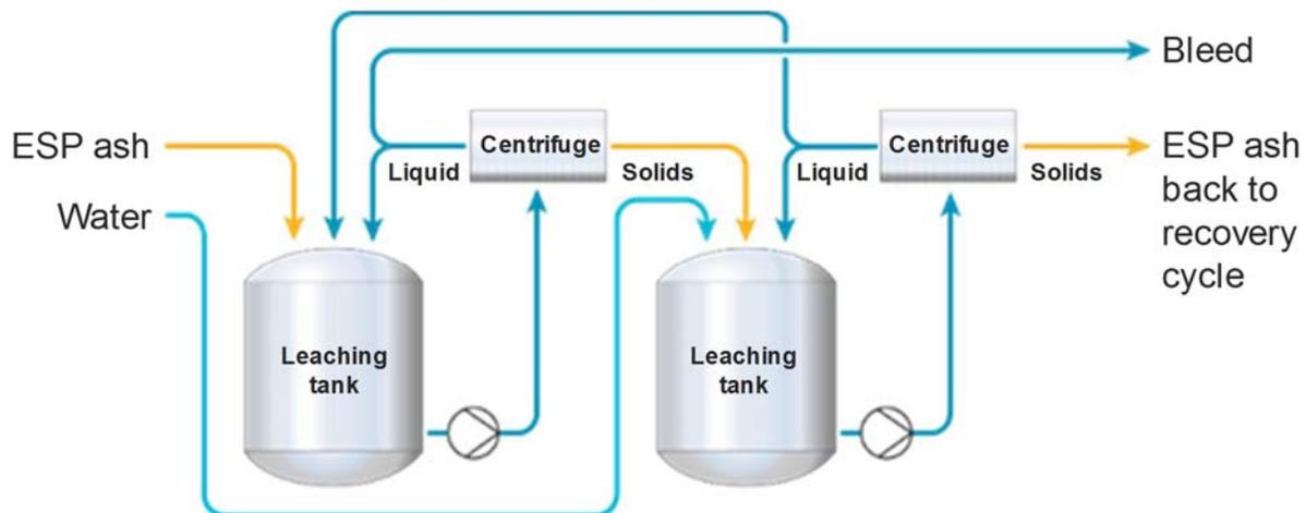
**Figure 9.** Ash leaching operation principle
