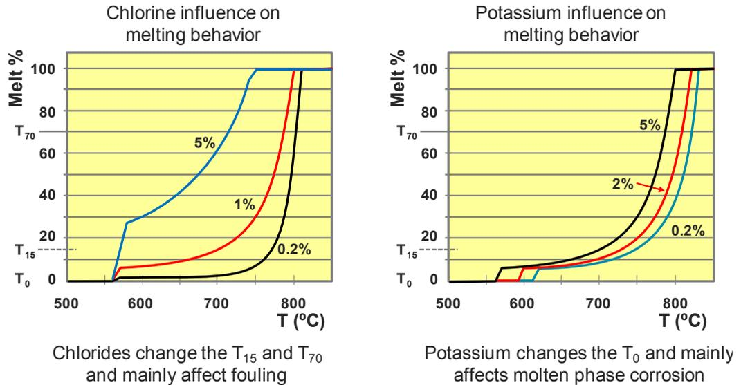
**Figure 7. Effect of K and Cl on corrosion and fouling**
