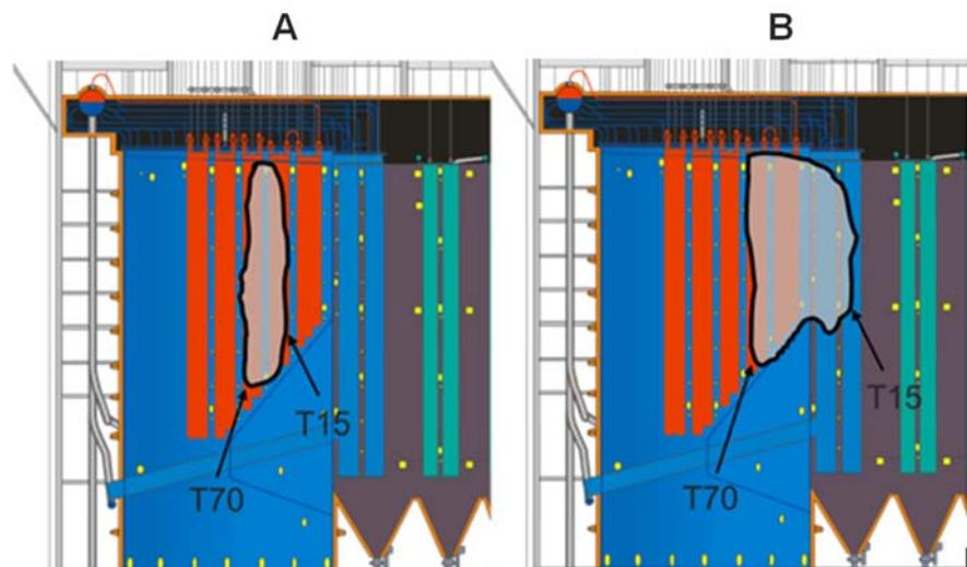
**Figure 8. Sticky area location with different K and Cl contents**
