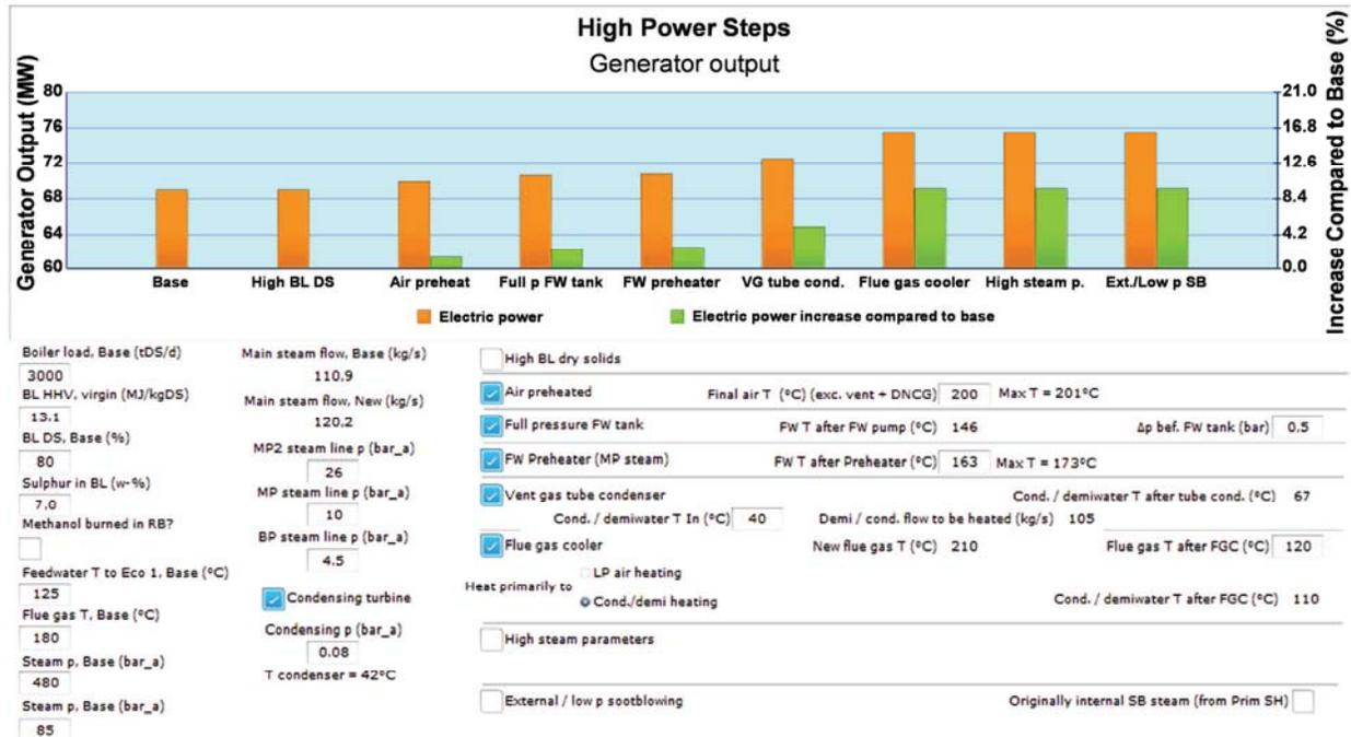
Figure 21. The effect of high power features on electricity production (Case study #1).
