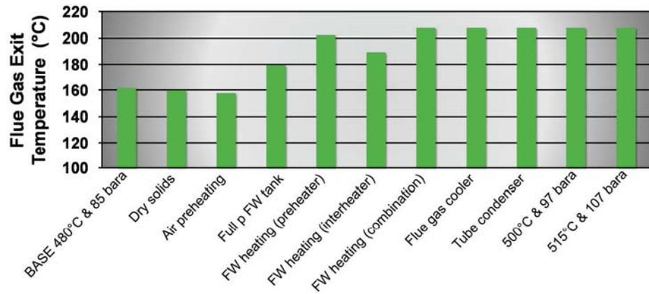
**Figure 19. Cumulative effect of high power features on flue gas exit temperature (FW = feedwater).**
