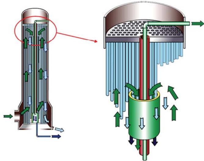
**Figure 9. Internal condensate segregation**
