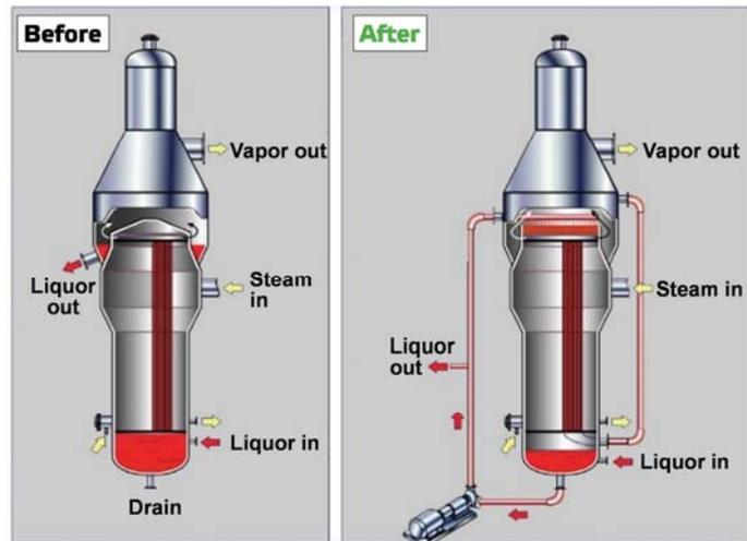
Figure 5. LTV to falling film conversion
