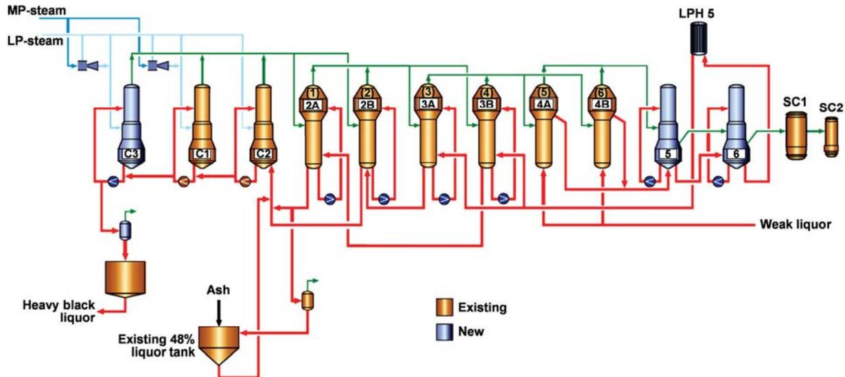
Figure 14. Eastern US mill revised evaporator arrangement
