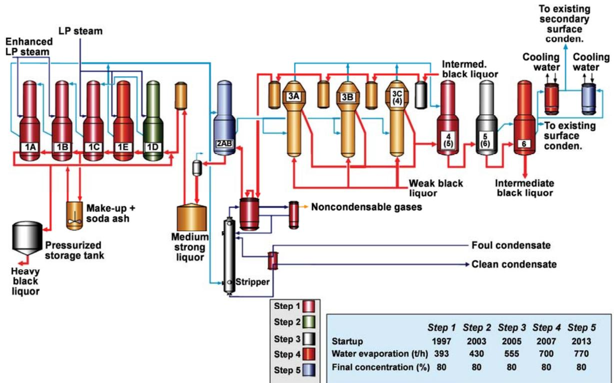
Figure 12. Klabin evaporator simplified flowsheet after 2013 upgrade
