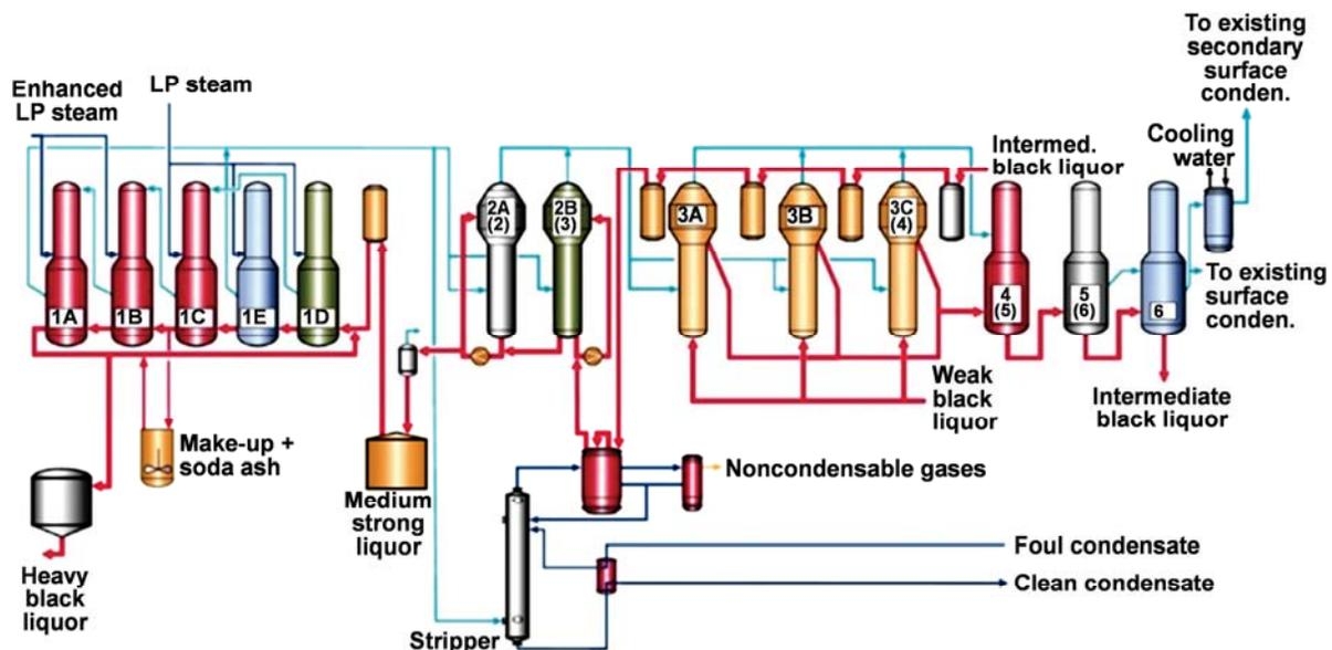
Figure 11. Klabin evaporator simplified flowsheet prior to 2013 upgrade
