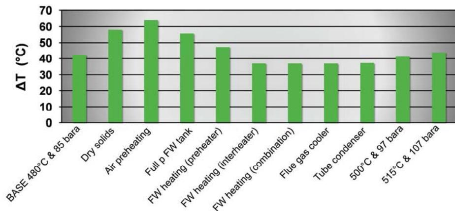
**Figure 18. Cumulative effect of high power features on temperature difference between drum and SWC (SWC = sweet water condenser; FW = feedwater).**
