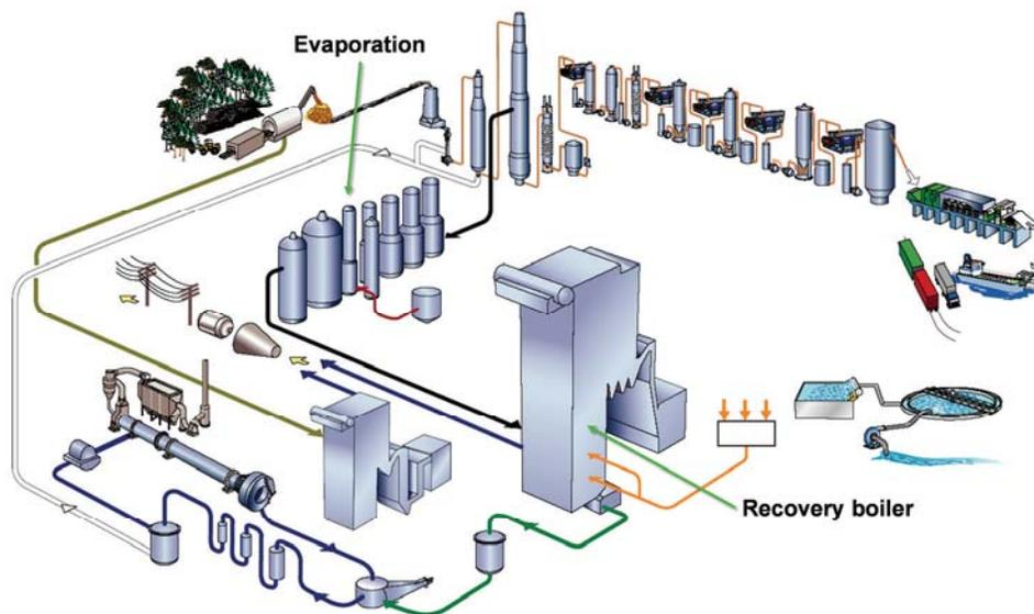
**Figure 2. Evaporator plant position in Kraft pulping**
