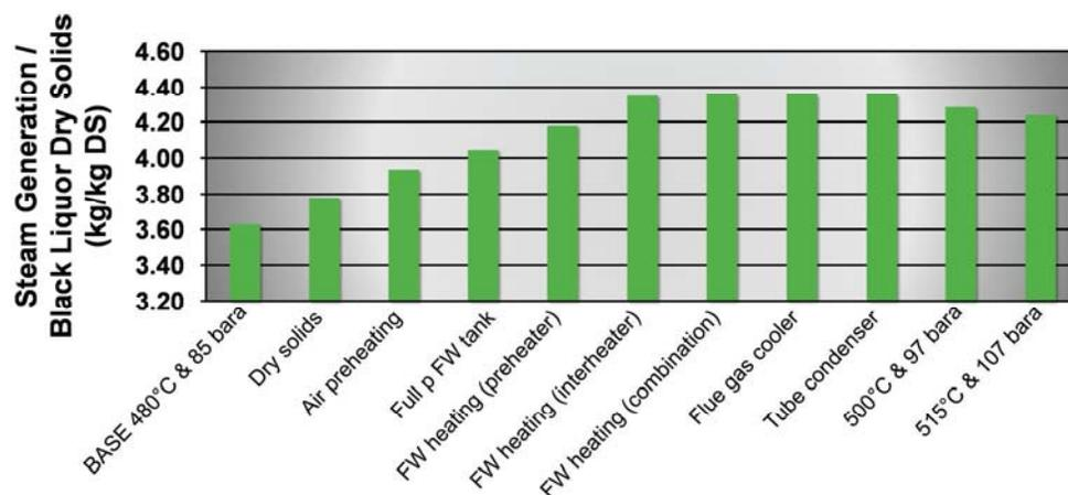
**Figure 16. Cumulative effect of high power features on the ratio of steam generation and black liquor dry solids (FW = feedwater).**
