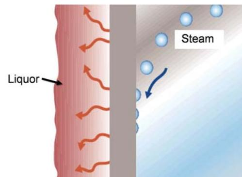
Figure 4. Falling film evaporation
