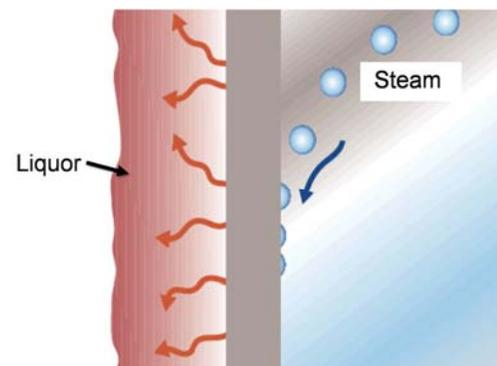
**Figure 4. Falling film evaporation**
