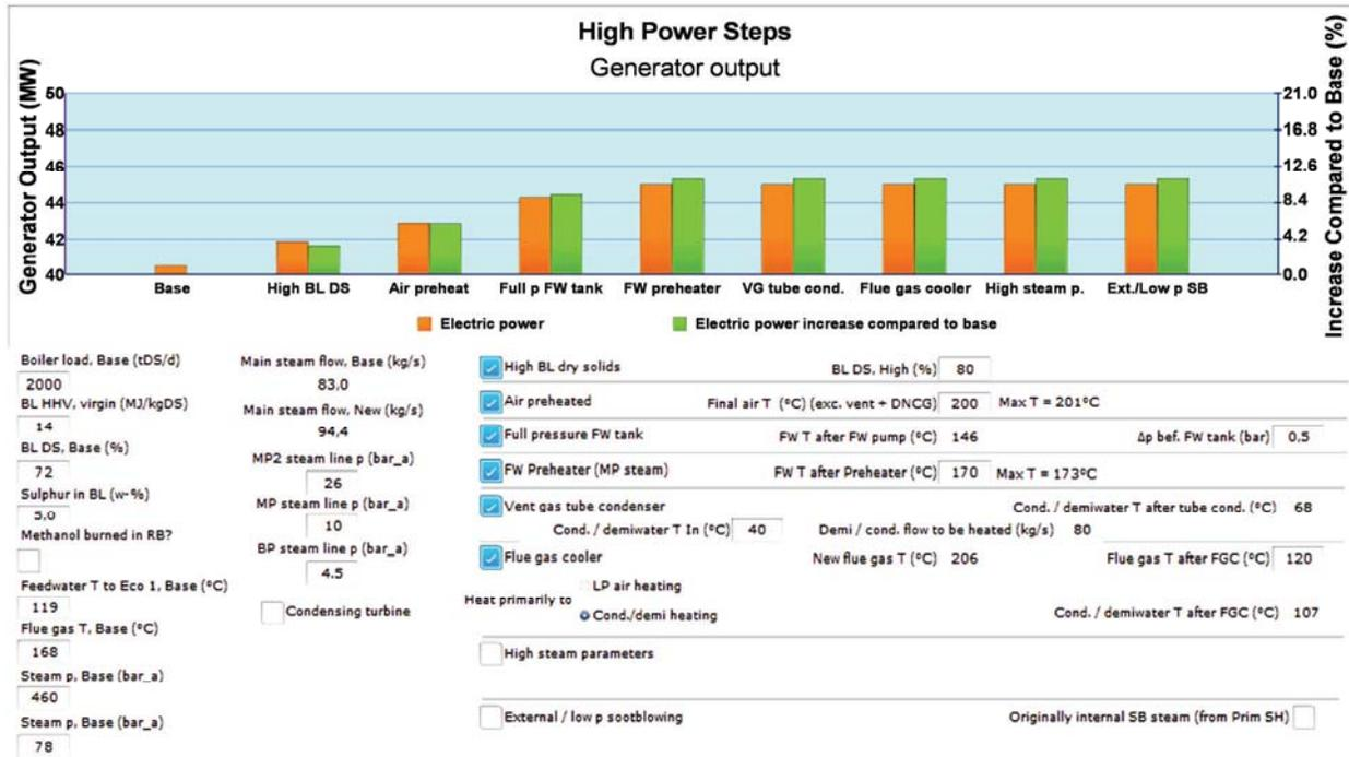
Figure 23. The effect of high power features on electricity production (Case study #2).
