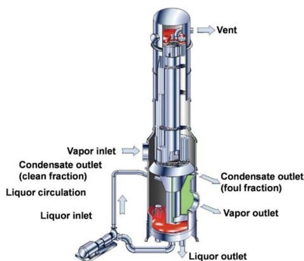
Figure 6. Conventional falling film
