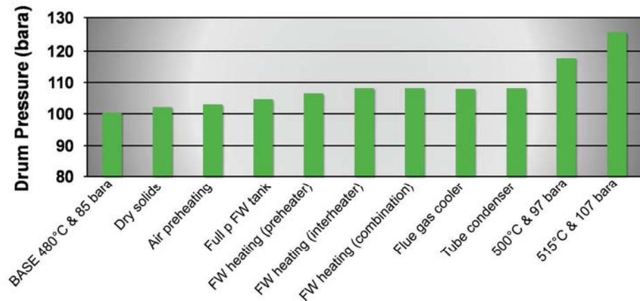
**Figure 20. Cumulative effect of high power features on drum pressure (FW = feedwater).**
