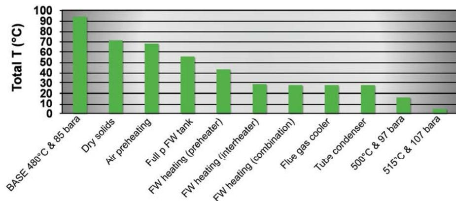
**Figure 17. Cumulative effect of high power features on total boiler steam attemperation (FW = feedwater).**
