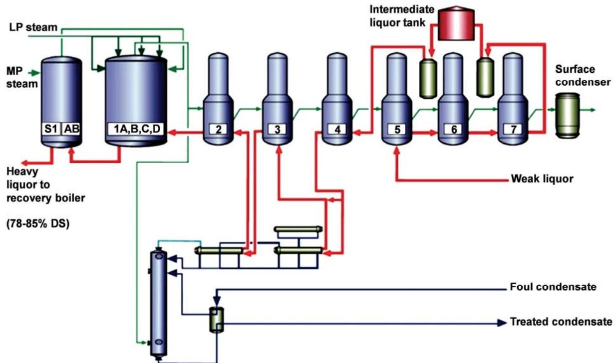
Figure 3. Simplified flow sheet for modern evaporators
