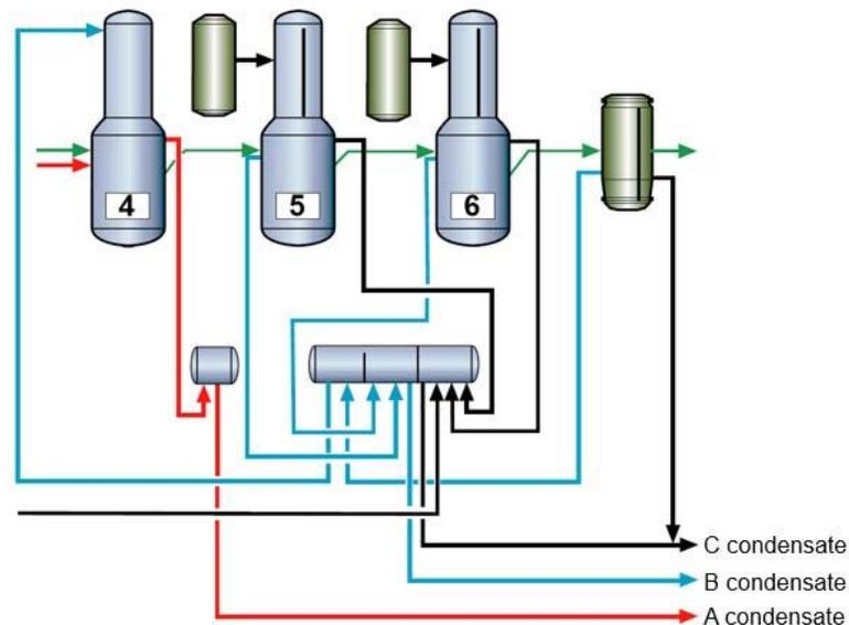
**Figure 10. Valmet's ICT processes a portion of the B-Condensate to make A-Condensate in the shell side of the 4<sup>th</sup> Effect.**
