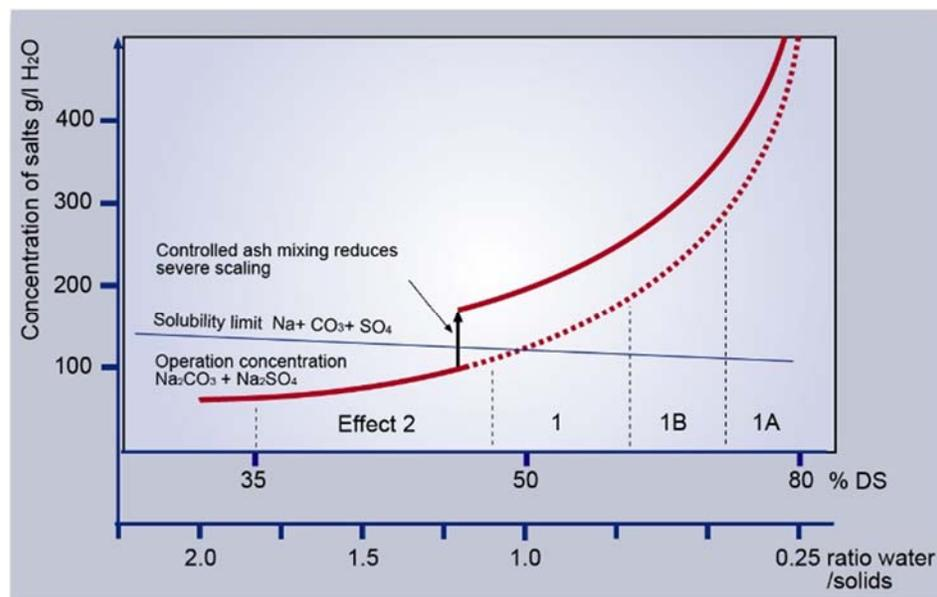
**Figure 4.** Recovery boiler ash mixing and heavy black liquor recirculation can avoid operation at the critical solids point.
