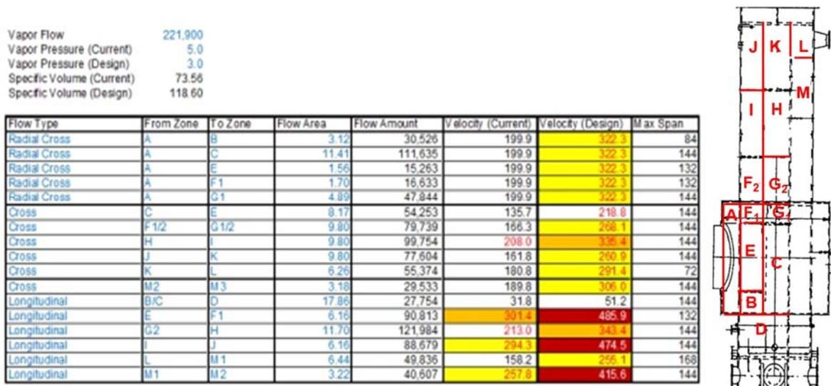
**Figure 8.** This typical condenser (right) is operating well past the design limits (shown in left chart as yellow, orange and red values). The result is vibration damage.
