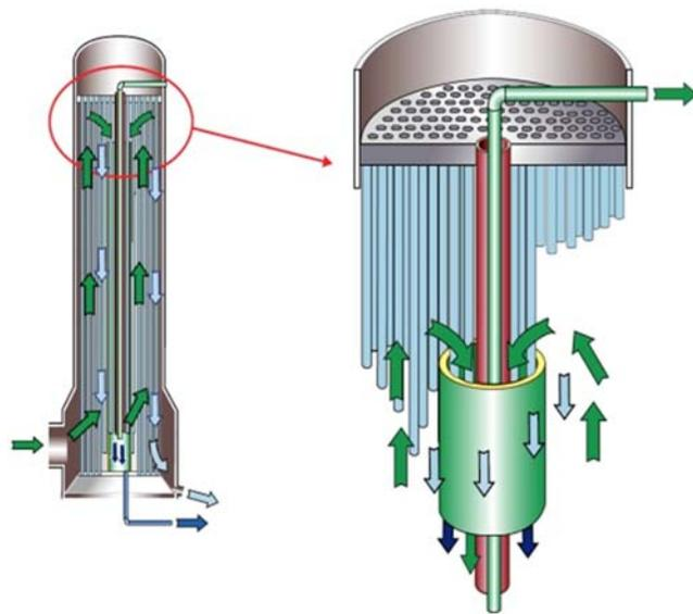
**Figure 9. Valmet's shell side design improves condensate segregation.**
