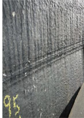
CS – In back-end effects, both shell and tube sides. Use 304L SS or Duplex Lite throughout
