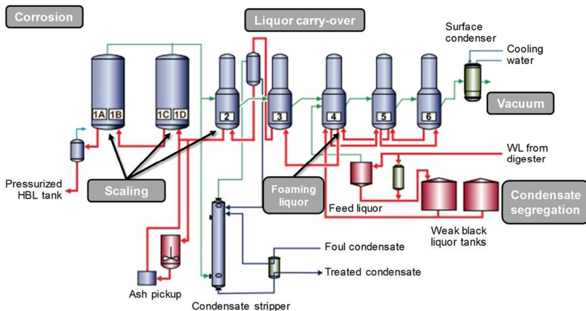
Figure 1. Problems inherent in the evaporator stage of the black liquor recovery process
