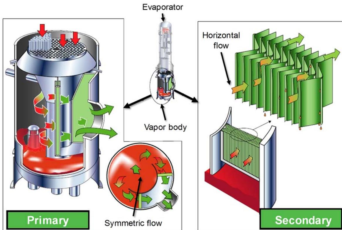
**Figure 7. Properly designed vapor body section with symmetric flow about the vapor outlet and horizontal flow through the chevrons.**
