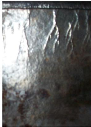
Tube thinning and SCC in concentrator units. Use Duplex above temperature threshold
