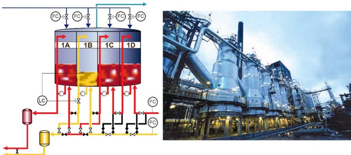
**Figure 5. CMPC Celulose Riograndense, Brazil has a completely new train with on-demand washing and REVAP Concentrator. Evaporation capacity: 430 tons/h, 75% DS product.**
