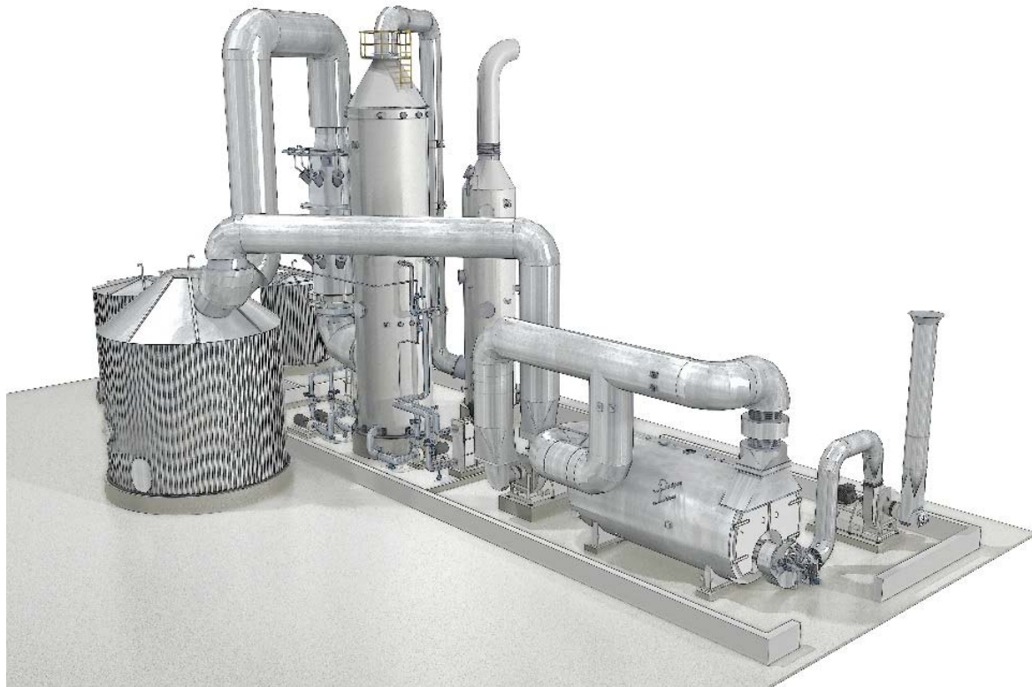
Figure 4: The sulfuric acid plant, based on the plant that is [being] built in the Metsä Fibre Äänekoski mill. The burner and boiler are located on the right, while the catalytic reaction vessel is located to the left in the image. The concentration tower and bisulfite scrubber are located to the right of the reaction vessel. The burner, boiler and the two towers are located inside a building (the lower part of the walls is seen in the image).
