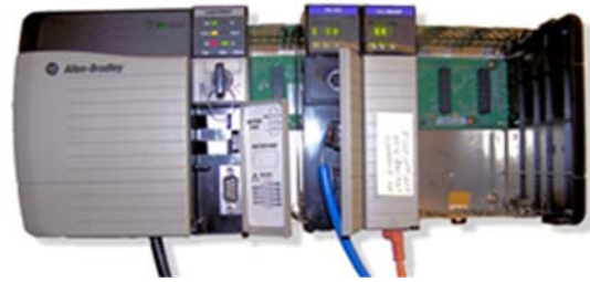
Figure 2. Parts are easily available for modern PLCs, such as this Allen-Bradley ControlLogix rack.
