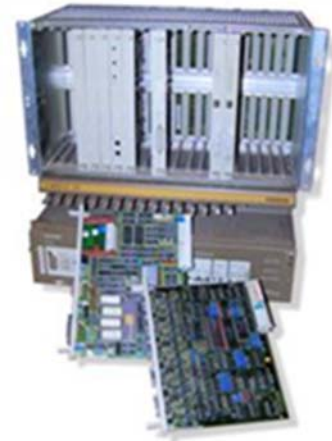
Figure 1. Obsolete PLC models, such as this Siemens S5-150U, may cause unexpected downtime for the entire machine line.
