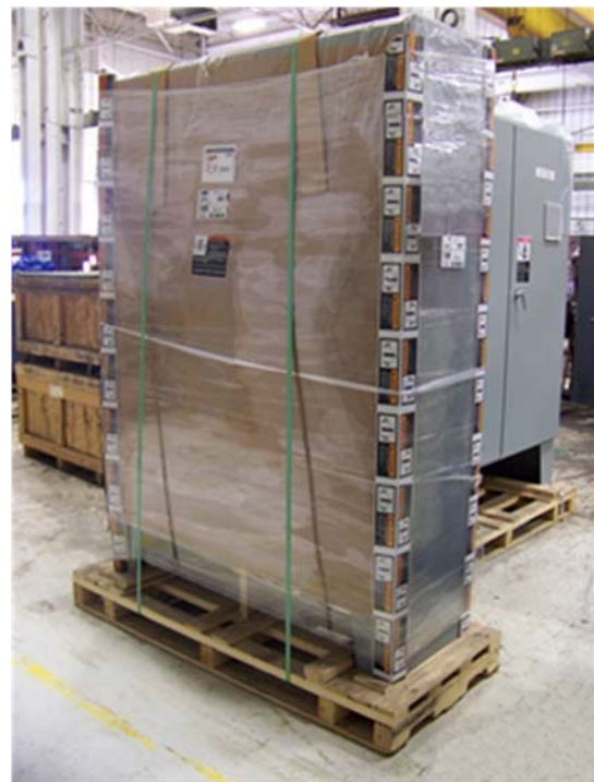
Figure 6. Two of many PLC cabinets on the Valmet workshop floor are ready to ship and be pre-installed at millsite. This can save considerable time on a short shutdown.
