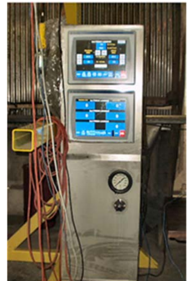
Figure 10. The operator local control station for the hydraulics controls upgrade is shown being fully tested on the Valmet workshop floor before shipment to the mill.
