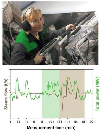
Figure 17. Energy efficiency analyses performed onsite can determine energy consumption at a paper machine, in this case total steam and electricity consumption.
