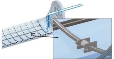
Figure 10. Valmet Dryer Cylinder Bars effectively break up the condensate layer inside the cylinder and produce a better heat transfer into the dryer shell.
