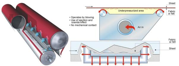
Figure 22. The Valmet Hirun Web Stabilizer blow box (left) operates without mechanical contact between the blow box and machine clothing.
