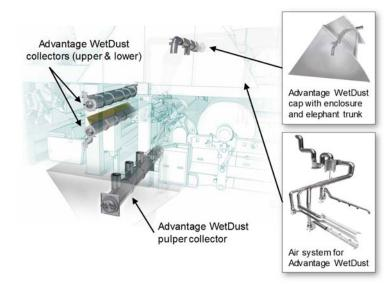
Figure 14. The Advantage WetDust innovative patented concept makes use of a fully wet system, eliminating typical issues associated with 'dry systems' (fires and plugging).
