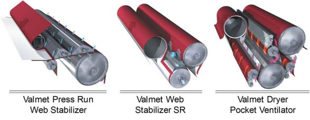
Figure 16. Careful selection and application of runnability components such as the Valmet Press Run Web Stabilizer and Valmet Web Stabilizer SR blow boxes and Valmet Dryer Pocket Ventilator can improve web stability while decreasing energy consumption.
