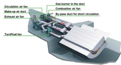
Figure 6. Valmet's TurnDry contactless dryer combines the TurnFloat air turn with the PowerDry air dryer to create a shorter drying layout and better runnability for coating machines. TurnDry air dryers simultaneously turn and dry the web during the sizing or coating drying process without touching the web itself.
