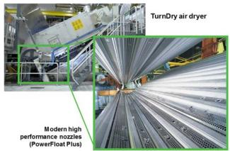
Figure 7. Valmet's patented PowerFloat Plus nozzles aren't just for new dryers such as the TurnDry shown here, but are also suitable as nozzle upgrades for old air dryers.
