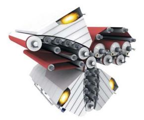
Figure 5. The OptiDry Twin impingement drying unit is designed to increase the dry content, and temperature, of paper at the beginning of the dryer section. This prevents sticking, strengthens the web and enables high speed.
