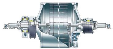
Figure 9. Valmet dryer internal view. Condensate removal can be arranged from one or both ends depending on cylinder size.
