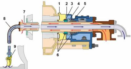
Figure 12. Spare parts for Beloit CS duplex steamfit with stationary syphon
