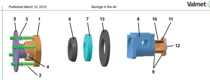
Figure 13. Replacement part kits for Beloit bellows duplex steamfit/syphon
