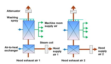
Figure 20. Flow sheet of the original Theresienthal heat recovery process.
