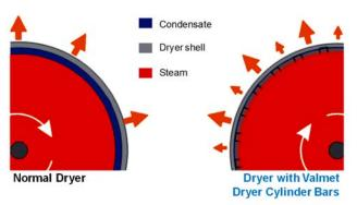
Figure 11. Comparison of heat flow through dryer shell (normal vs. Valmet Dryer Cylinder Bars ).
