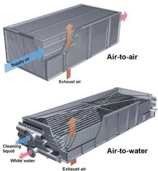
Figure 4. Not all heat recovery is created equal. Air-to-air (top) is custom designed with wide plate spacing, minimal pressure drop and high efficiency. Air-to-water (bottom) is a squat design using individual tubes and minimal welds for a modular approach.
