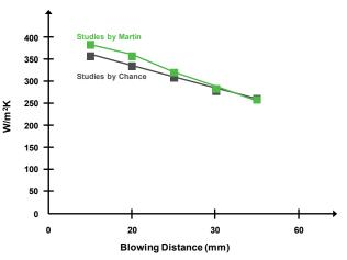
Figure 9. Heat transfer coefficient change as a function of impingement distance.
