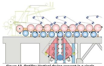
Figure 13. OptiDry Vertical drying concept in a singlefelted drying section rebuild
