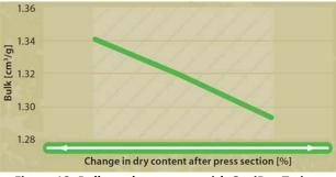
Figure 18. Bulk vs. dry content with OptiDry Twin on pilot machine
