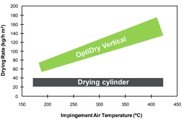
*Figure 3. Evaporation rate achieved using OptiDry impingement drying. Pilot machine tests.*
