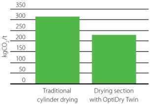
Figure 25. CO<sub>2</sub> emission comparison of traditional vs. OptiDry drying (steam is generated by coal)
