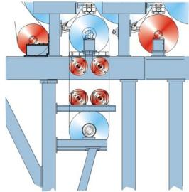
Figure 10. Vertical geometry OptiDry on Valmet pilot machine #2 (2004)
