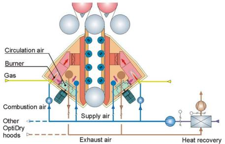
Figure 11. Air system for OptiDry Vertical impingement drying unit
