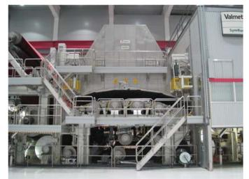
Figure 15. The OptiDry Curl installed at Propapier PM2 (2010 startup) is used for curl control at the end of the after-dryer section. The steam heated dryer can be changed to gas heated. The circulation air fan and steam coil are located outside the dryer.
