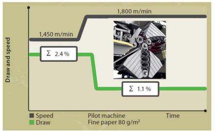
Figure 17. Significant draw reduction with OptiDry Twin on pilot machine
