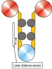
Figure 7. Vertical geometry OptiDry unit on Valmet's pilot machine #1 in Rautpohja, Finland.
