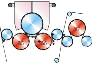
Figure 2. OptiDry impingement drying at Valmet's pilot machine #2 (1995)
