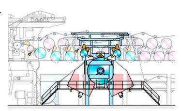
*Figure 4. OptiDry impingement drying unit on a production machine (1999)*
