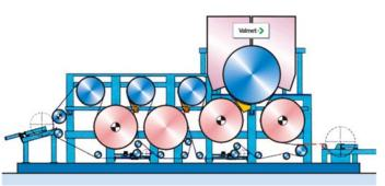
Figure 1. Impingement drying pilot unit in Jyväskylä, Finland (1993).
