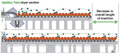
Heat recovery from the exhaust air in OptiDry Twin drying is significantly more effective than in cylinder drying due to the higher temperature and humidity of the exhausted air. The heat energy recovered from the exhaust air is about 12.3 MW in the case of the OptiDry concept, compared with about 8.3 MW in the case of a cylinder configuration.
