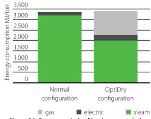
Figure 24. Energy analysis of impingement drying vs. normal single-felted cylinder drying in a predryer section
