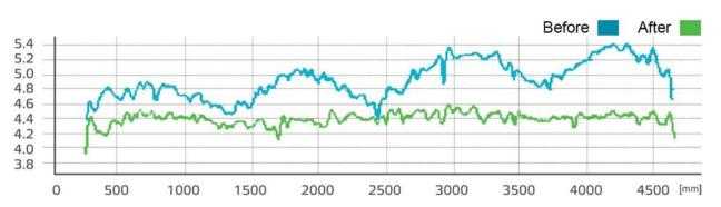
Figure 24. Stora Enso Kemi experienced significantly improved moisture profiles at the reel after the installation of OptiDry Profile on CM1.
