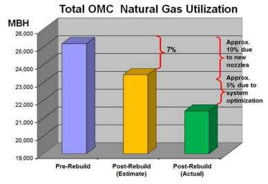
Figure 6. Energy savings with new air bars
