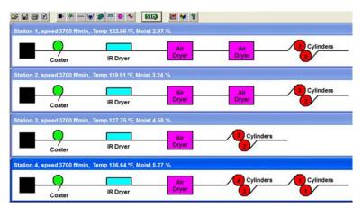
Figure 4. Computer model of off-machine coater
