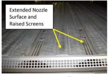
Figure 15. New air bars (flotation nozzles) and screens (post-rebuild)
