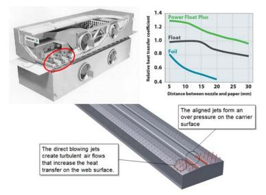
Figure 18. Valmet Air Dryer Nozzles increase drying effectiveness
