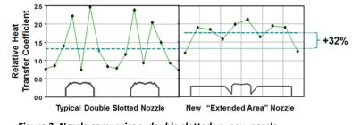
Figure 3. Nozzle comparison: double slotted vs. new nozzle
