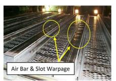
Figure 13. Warped bars (pre-rebuild) and return screens
