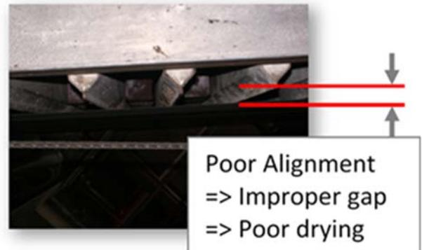
Figure 1. Typical air bar to web alignment
