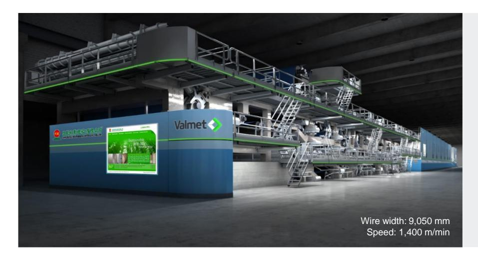
Six containerboard making lines with modern industrial design. In addition to increasing safety and usability, the board machines are also very energy and resource efficient and suitable for high-speed production.
