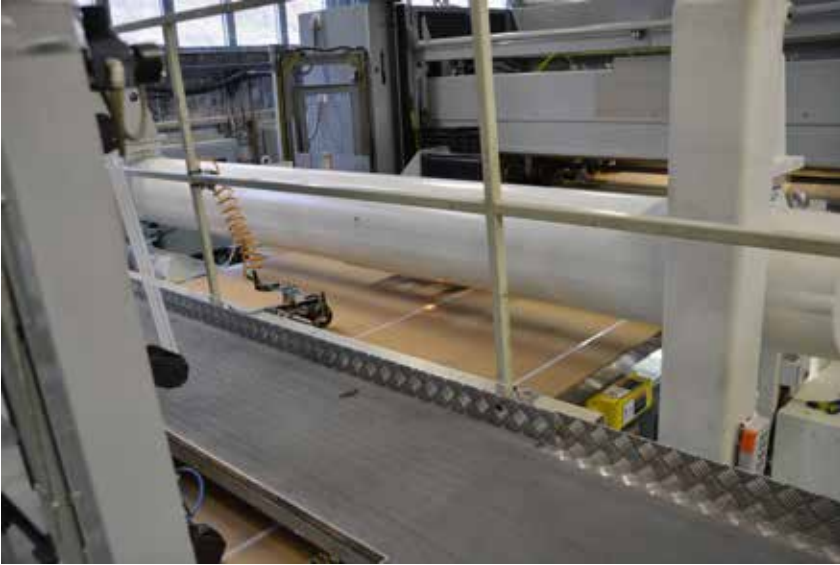
THE IQ SCANNER MEASURES THE SURFACE MOISTURE ACROSS THE CORRUGATED BOARD WEB.
