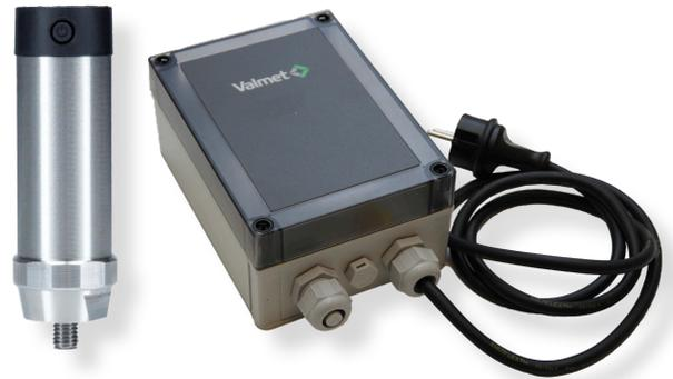
WVS-200 is an industrial wireless vibration sensor for mechanical condition monitoring. It has built-in MEMS-accelerometer and temperature sensor. WVS-200 provides a cost-efficient monitoring solution for non-critical machinery or as an alternative for route-based condition monitoring.
